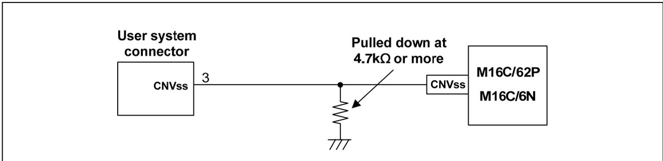
Figure 5.10 E8a Emulator and CNVss Pin Connection
