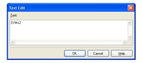
Enter the macro definition in the format of "macro name=defined value", with one macro name per line. You can specify up to 31 characters per line, up to 30 line. The "=defined value" part can be omitted, and in this case, "1" is used as the defined value.
