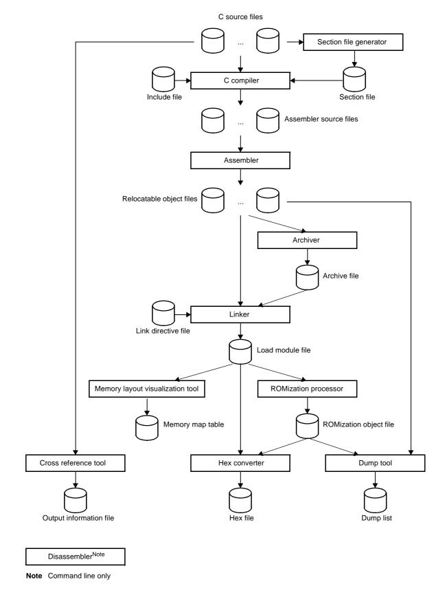
Figure 1-1. Build Tool Process Flow
