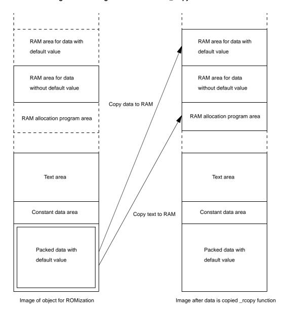
Figure B-27. Image of Before and After \_rcopy Function Is Called
