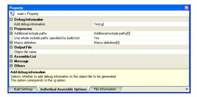
You can set assemble options for the assembler source file by setting the necessary properties in this tab. Note that this tab takes over the settings of the [Assemble Options] tab by default.
