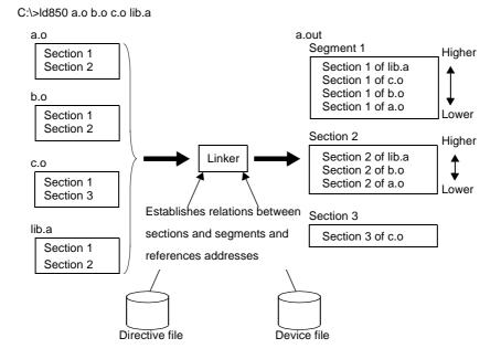
The ca850 internally activates the as850 and linker as drivers.
