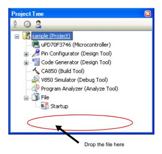
Caution To add other than a startup routine, drop a file onto the Startup node. See "2.3.1 Set a startup routine" for details about using other than a startup routine.
