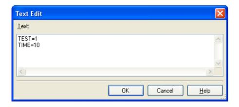
Enter the macro definition in the format of "macro name=defined value", with one macro name per line. You can specify up to 256 characters per line, up to 30 line. The "=defined value" part can be omitted, and in this case, "1" is used as the defined value.
