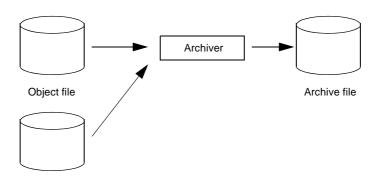
The archive file generated by the archiver can be specified as an input file to the linker. If an archive file is specified, the ld850 searches the necessary objects from the specified archive file, and links only the objects found.
