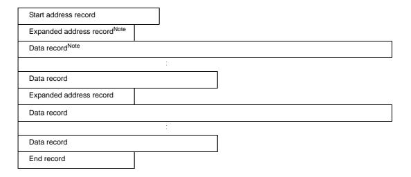
Note The expanded address record and data record are repeated.
