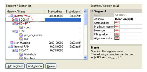
Figure 2-7. Section Detail (When .sconst Is Selected)
