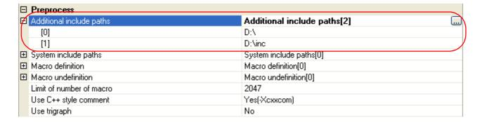
To change the include paths, you can use the [...] button or enter the path directly in the text box of the subproperty. When the include path is added to the project tree, the path is added to the top of the subproperties automatically.
