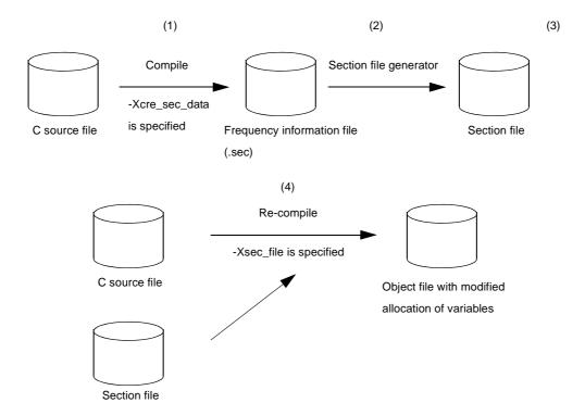
Figure B-40. Image of Compilation Using Section File Specifications
