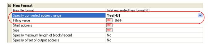
Enter the fill value for the vacant area directly to the text box. The range that can be specified for the value is 0x00 to 0xFF (hexadecimal). "0xFFFF" is set by default.
