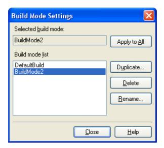
If you select the build mode to be changed from the build mode list, the selected build mode is displayed in [Selected build mode]. If you click the [Apply to All] button, the build mode for the main project and all the subprojects which belong to the project will be changed to the build mode selected in the dialog box.
