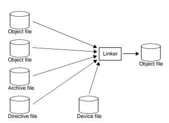
Figure B-8. Operation Flow of Linker
