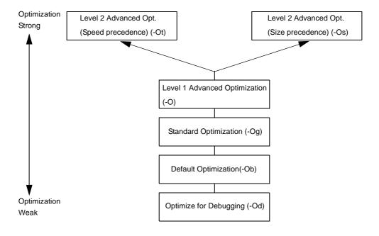
Figure B-3. Optimization Processing and Parameters
