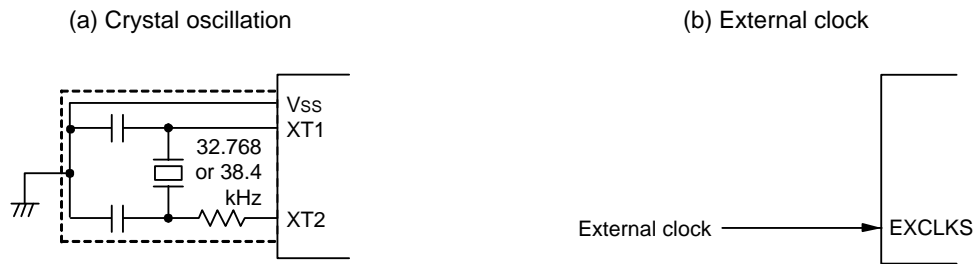
Figure 6-21. Example of External Circuit of XT1 Oscillator
