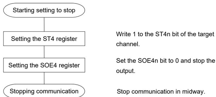
**Remark** Even after communication is stopped, the pin level is retained. To resume the operation, re-set serial output register 4 (SO4) (see **Figure 16-54 Procedure for Resuming DALI Transmission**).
