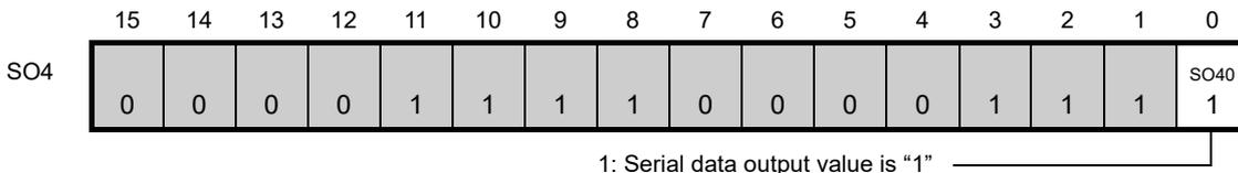
(h) Serial output enable register 4 (SOE4) ... Sets only the bits of the target channel to 1.
