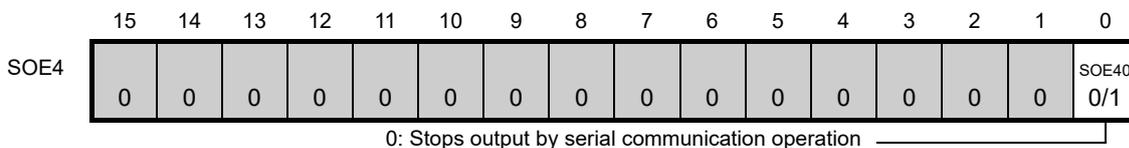
\* For channel n, whose serial output is stopped, the SO4n bit value of the SO4 register can be set by software.
