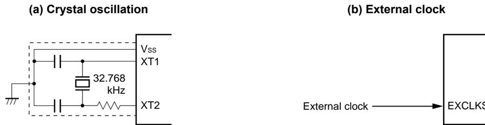
**Caution** When using the X1 oscillator and XT1 oscillator, wire as follows in the area enclosed by the broken lines in the Figures 5-14 and 5-15 to avoid an adverse effect from wiring capacitance.
