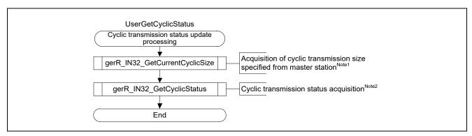
Figure 4.12Flowchart for Cyclic Transmission Status Update Processing
