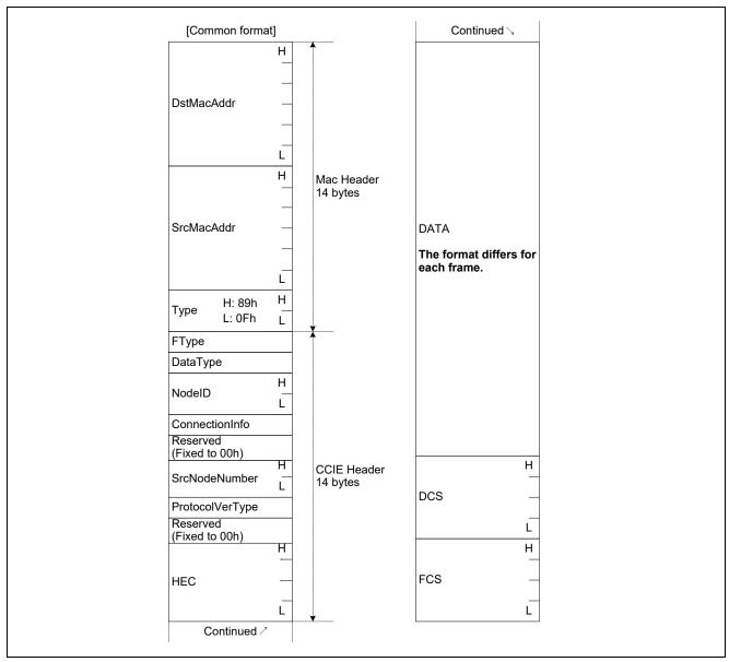
Figure 7.1 Overview of Frame Common Format
