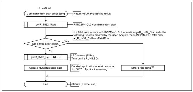
Figure 4.3 Flowchart for Communication Start Processing
