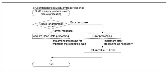
Figure 4.36Flowchart for SLMP Memory Read Response Receive Processing
