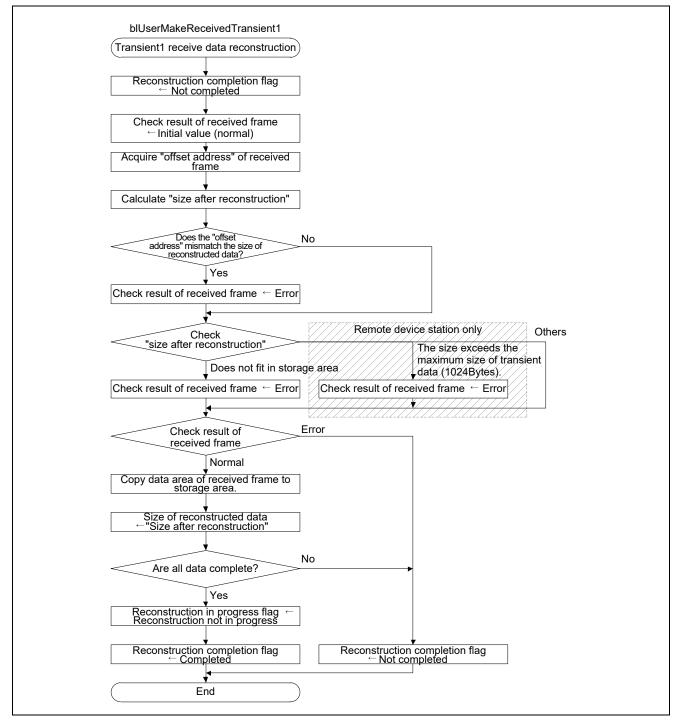
Figure 4.21Flowchart for Transient1 Receive Data Reconstruction Processing
