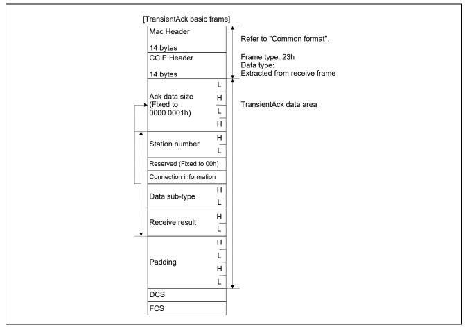
Figure 7.17Overview of TransientAck Frame Format
