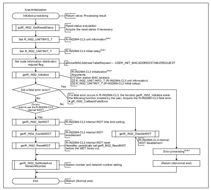
Figure 4.2 Flowchart for Initialization Processing
