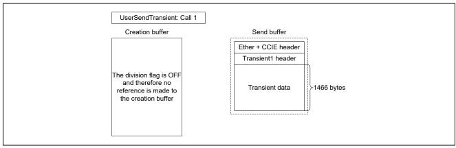
Figure 4.32When Dividing and Transferring Transient Data Having a Size of 1466 Bytes or Less (When the Division Flag is OFF)
