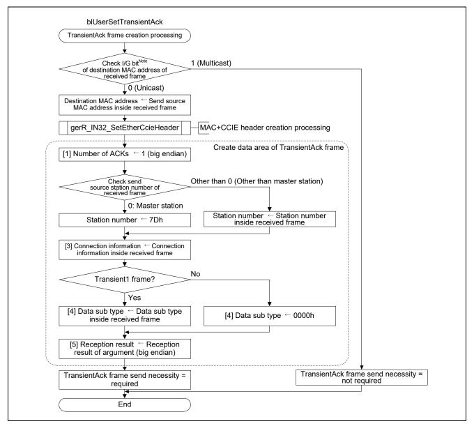
Figure 4.29Flowchart for TransientAck Frame Creation Processing
