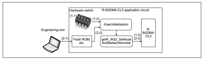
Figure 2.2 Image of Setting Station Number and Network Number
