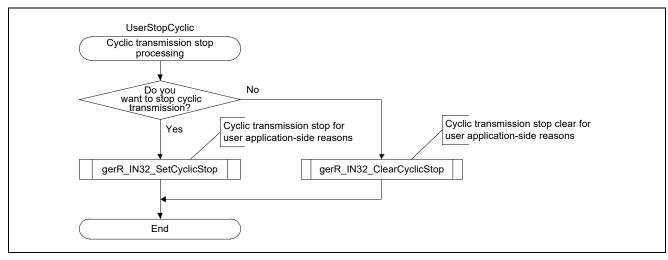
Figure 4.5 Flowchart for Cyclic Transmission Stop Processing
