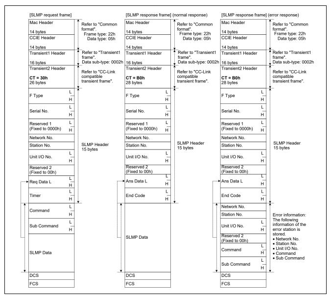
Figure 7.14Overview of SLMP Frame Basic Format
