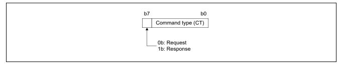
Figure 7.5 Data Structure of CC-Link Compatible Transient Command Type
