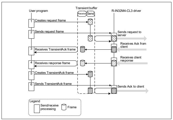
Figure 4.15Client Processing Procedure
