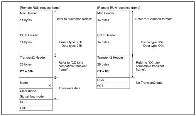
Figure 7.8 Overview of Remote RUN Frame Format
