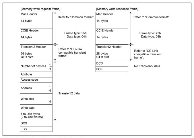
Figure 7.11Overview of Memory Write Frame Format
