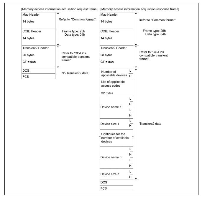
Figure 7.6 Overview of Memory Access Information Acquisition Frame Format
