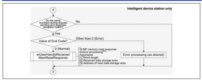
Figure 4.17Flowchart for Transient1 Receive Data Processing (4/4)
