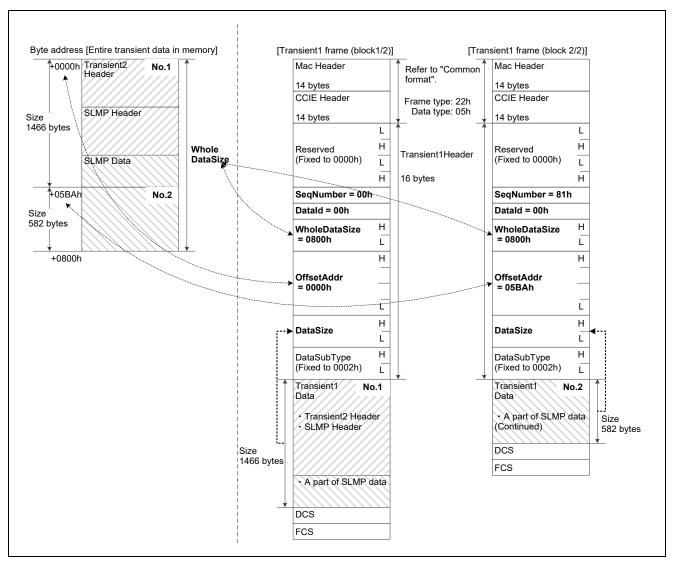
Figure 7.3 Example of Transient1 Frame Division
