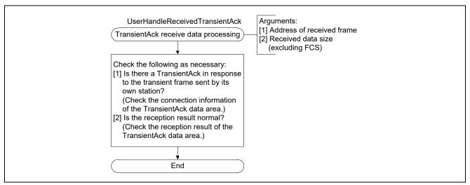
Figure 4.28Flowchart for TransientAck Receive Data Processing
