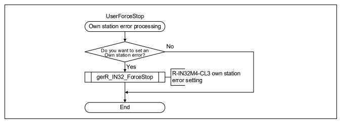
Figure 4.4 Flowchart for Own Station Error Processing
