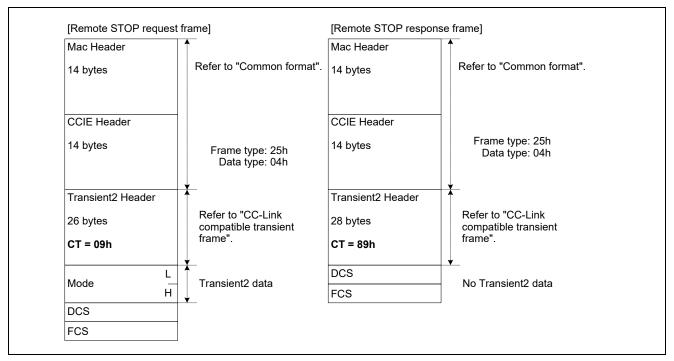
Figure 7.9 Overview of Remote STOP Frame Format
