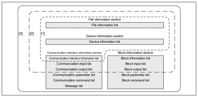
Figure 2.3 CSP+ File Section Configuration
