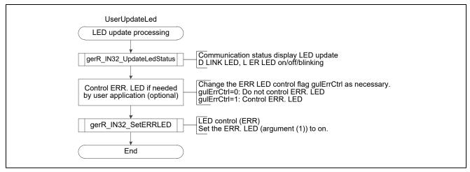
Figure 4.11Flowchart for LED Update Processing
