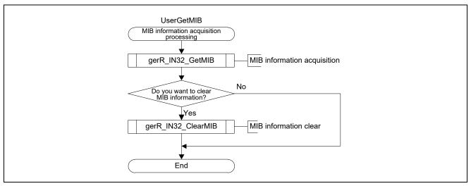
Figure 4.13Flowchart for MIB Information Acquisition Processing
