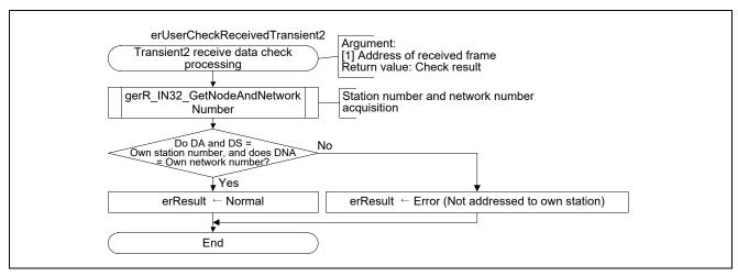
Figure 4.25Flowchart for Transient2 Receive Data Check Processing
