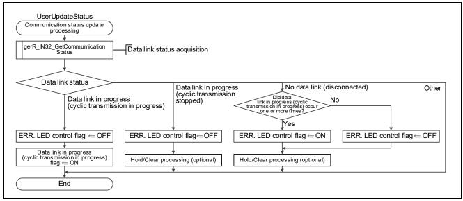
Figure 4.10Flowchart for Communication Status Update Processing
