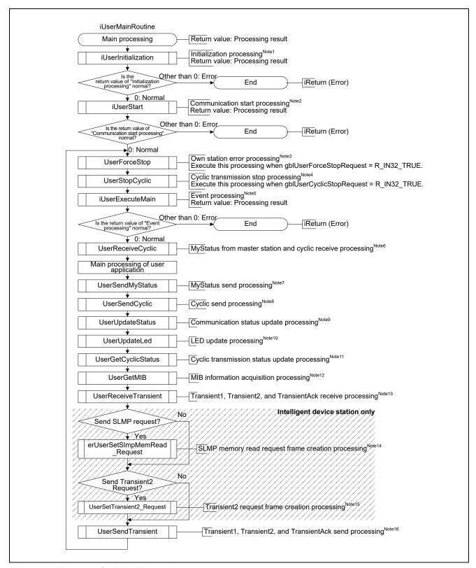
Figure 4.1 Flowchart for Main Processing
