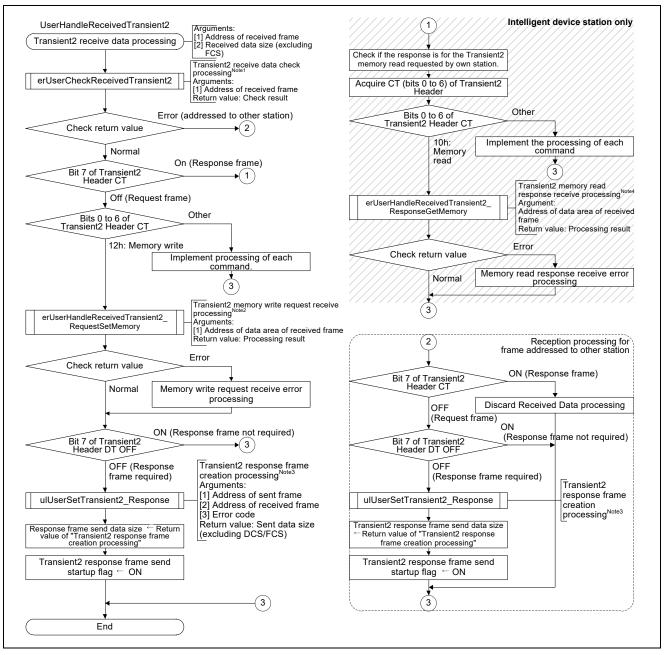
Figure 4.24Flowchart for Transient2 Receive Data Processing
