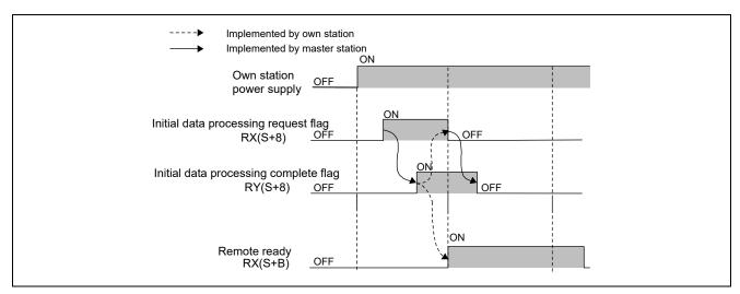
Figure 6.2 Timing Chart: Initial Data Processing Request/Complete Flag
