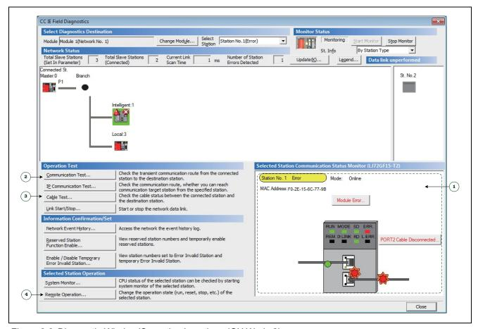
Figure 3.6 Diagnostic Window/Operation Locations (GX Works2)
