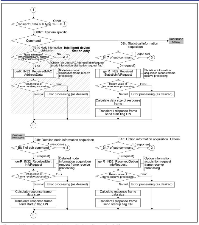
Figure 4.17Flowchart for Transient1 Receive Data Processing (2/4)
