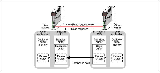
Figure 3.4 Flow of Transient Data
