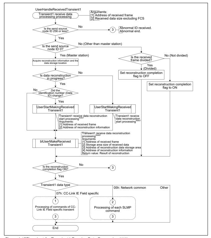
Figure 4.17Flowchart for Transient1 Receive Data Processing (1/4)
