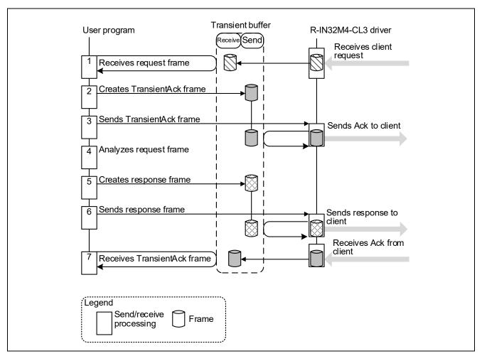
Figure 4.14Server Processing Procedure
