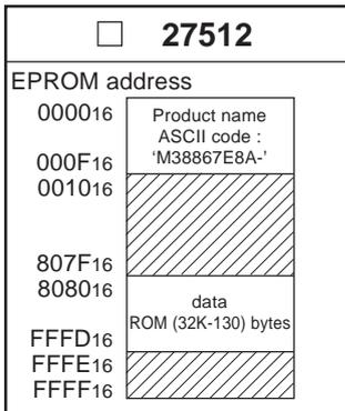
In the address space of the microcomputer, the internal ROM area is from address 8080<sub>16</sub> to FFFD<sub>16</sub>. The reset vector is stored in addresses FFFC<sub>16</sub> and FFFD<sub>16</sub>.
