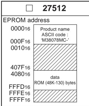
In the address space of the microcomputer, the internal ROM area is from address 4080<sub>16</sub> to FFFD<sub>16</sub>. The reset vector is stored in addresses FFFC<sub>16</sub> and FFFD<sub>16</sub>.
