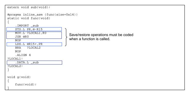
A C source file that includes assembly functions must be output in an assembly file format (code=asmcode).
