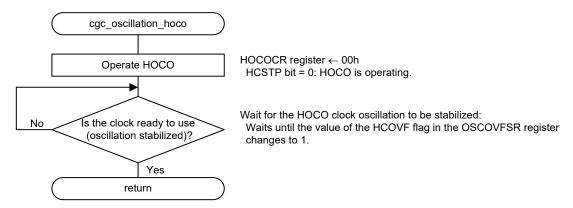
Figure 3.6 HOCO Clock Oscillation Setting
