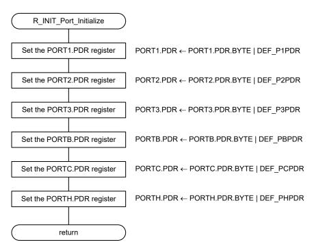
Figure 3.3 Nonexistent Port Initialization
