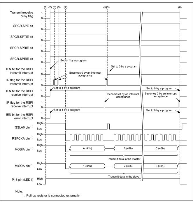
Figure 7.2 Timing of Serial Communication with SPI Operation (Four-Wire Method)
