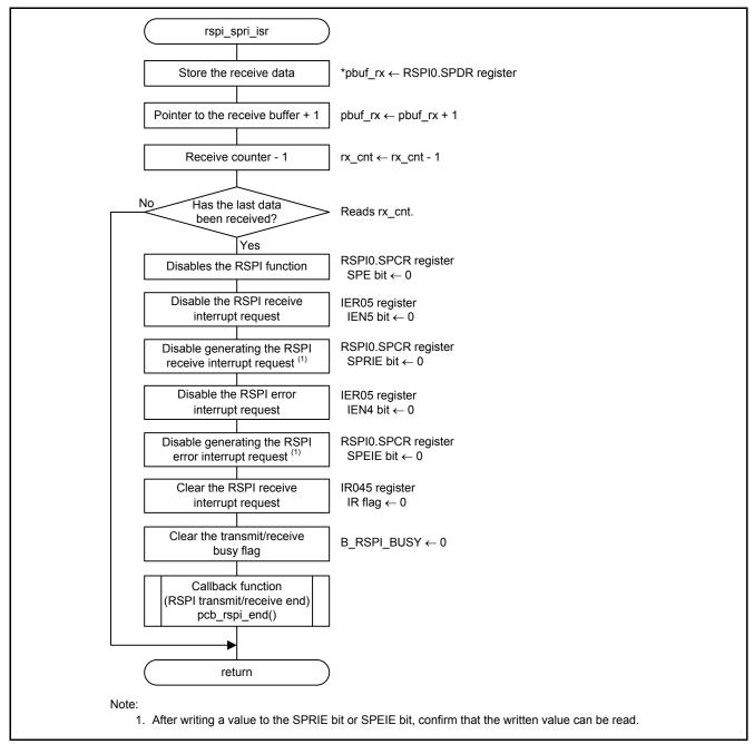
Figure 7.15 RSPI Receive Interrupt
