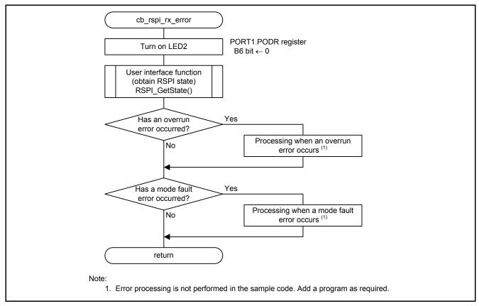
Figure 7.8 Callback Function (RSPI Receive Error)
