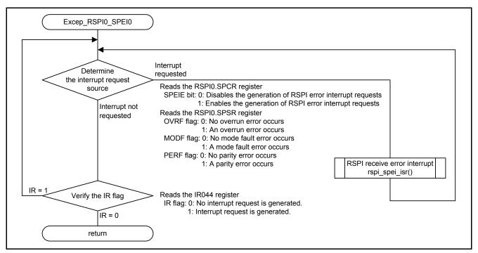
Figure 7.17 RSPI0.SPEI0 Interrupt Handling
