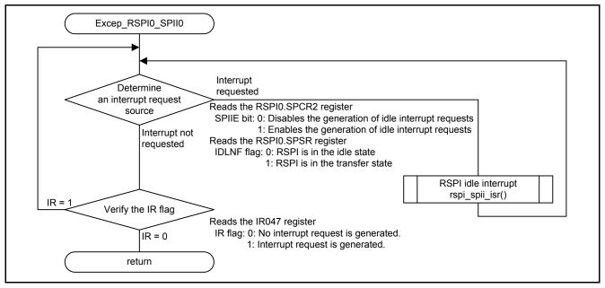
Figure 5.23 RSPI0.SPII0 Interrupt Handling
