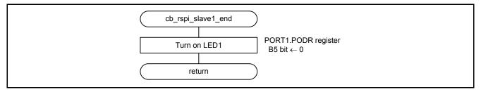
Figure 5.9 Callback Function (Completion of RSPI Transmission to/Reception from Slave 1)
