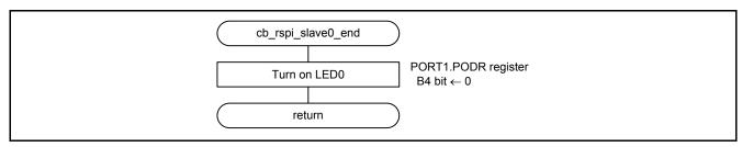
Figure 5.8 Callback Function (Completion of RSPI Transmission to/Reception from Slave 0)
