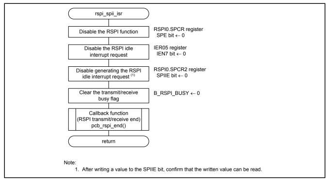
Figure 5.17 RSPI Idle Interrupt
