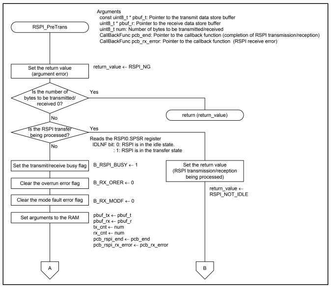
Figure 7.11 User Interface Function (RSPI Transmit/Receive Start) (1/2)
