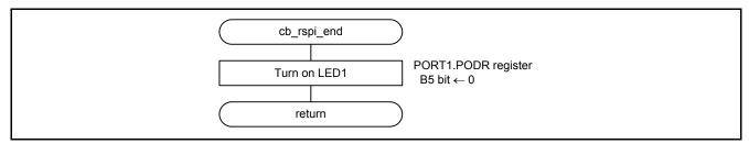
Figure 7.7 Callback Function (Completion of RSPI Transmission to/Reception from the Master)
