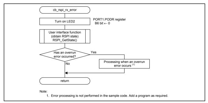
Figure 5.10 Callback Function (RSPI Receive Error)
