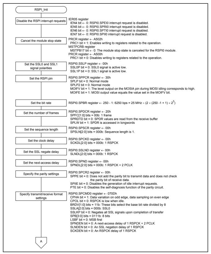
Figure 5.11 User Interface Function (RSPI Initialization) (1/2)
