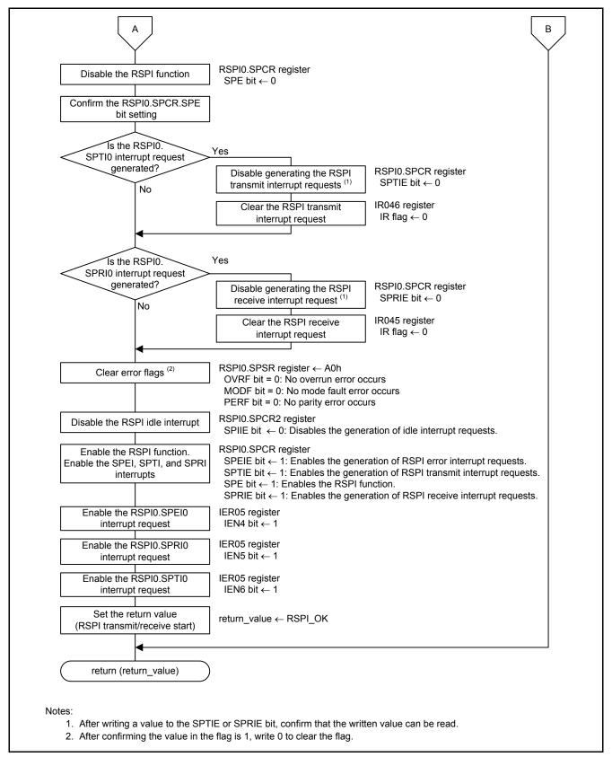
Figure 7.12 User Interface Function (RSPI Transmit/Receive Start) (2/2)
