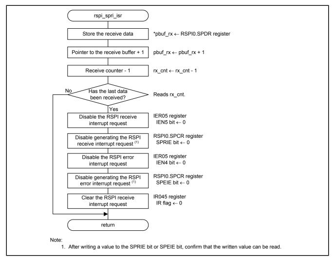
Figure 5.18 RSPI Receive Interrupt
