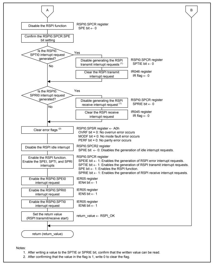
Figure 5.14 User Interface Function (RSPI Transmit/Receive Start) (2/2)
