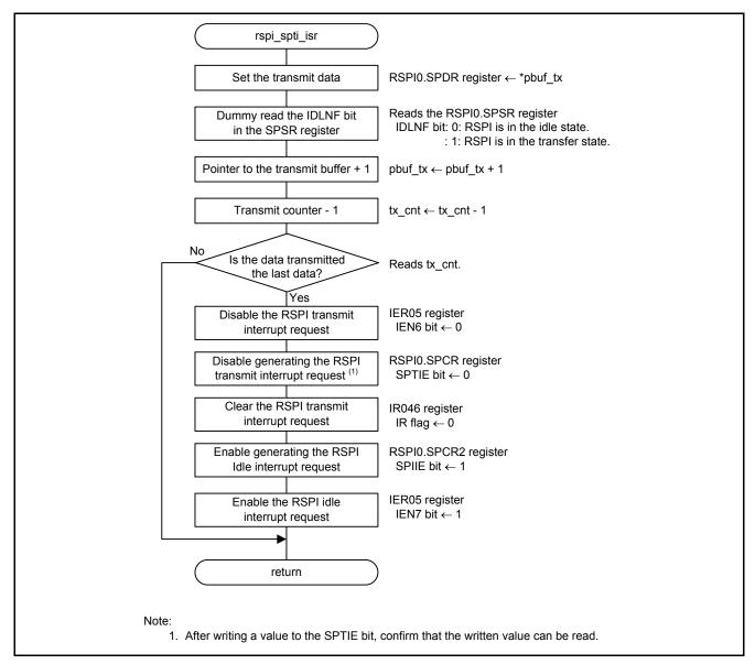
Figure 5.16 RSPI Transmit Interrupt
