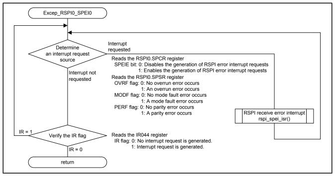
Figure 5.20 RSPI0.SPEI0 Interrupt Handling
