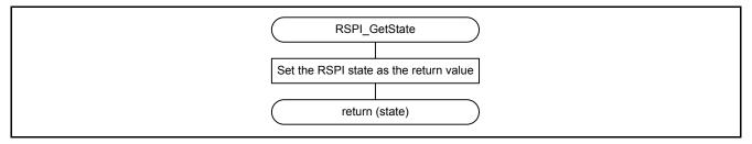
Figure 5.15 User Interface Function (Obtain RSPI State)
