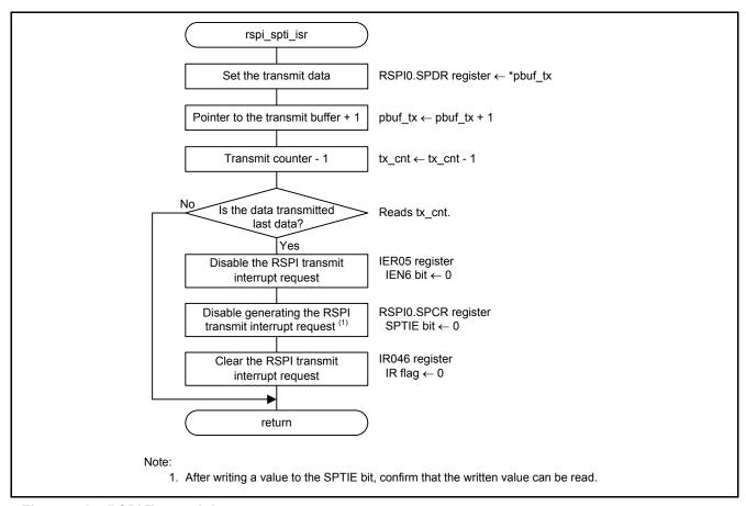
Figure 7.14 RSPI Transmit Interrupt
