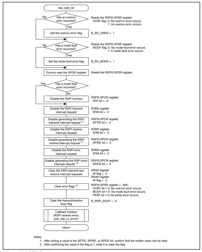
Figure 7.16 RSPI Error Interrupt
