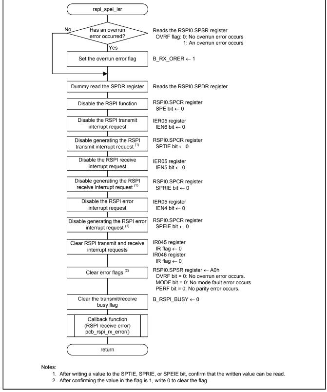
Figure 5.19 RSPI Error Interrupt
