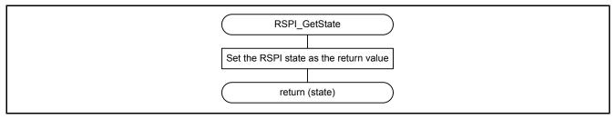
Figure 7.13 User Interface Function (Obtain RSPI State)
