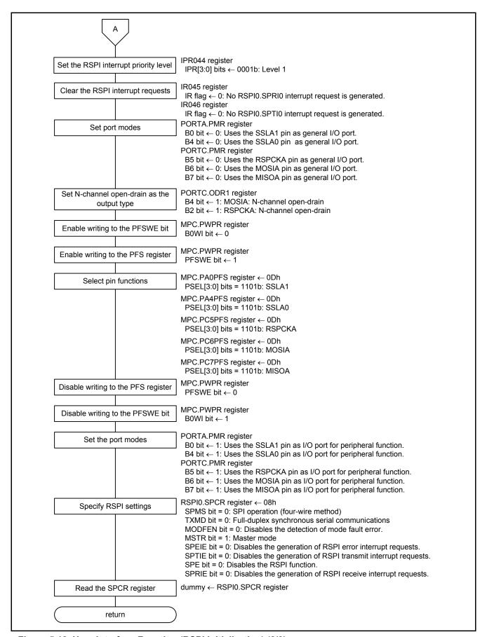
Figure 5.12 User Interface Function (RSPI Initialization) (2/2)
