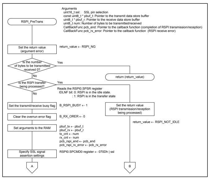
Figure 5.13 User Interface Function (RSPI Transmit/Receive Start) (1/2)
