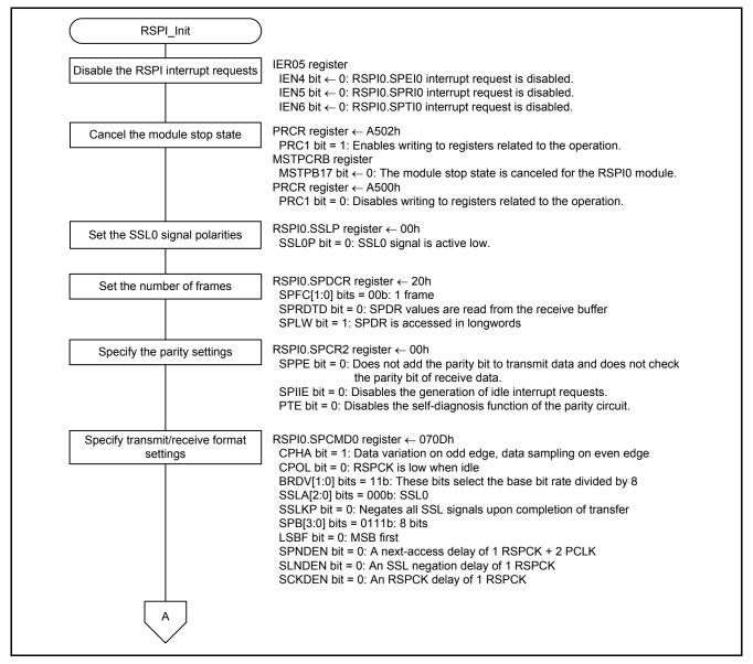
Figure 7.9 User Interface Function (RSPI Initialization) (1/2)
