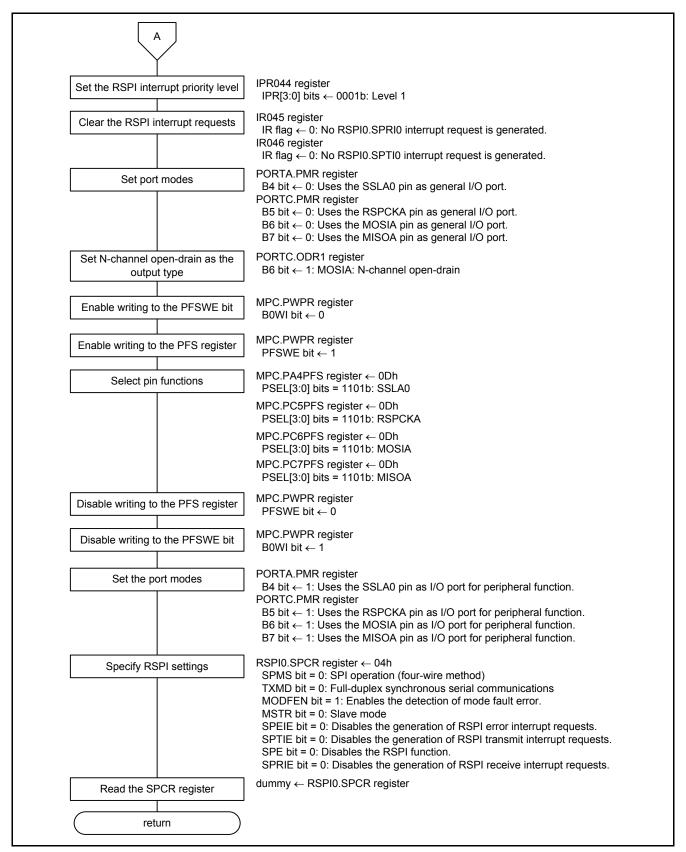
Figure 7.10 User Interface Function (RSPI Initialization) (2/2)
