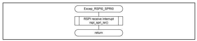
Figure 5.21 RSPI0.SPRI0 Interrupt Handling
