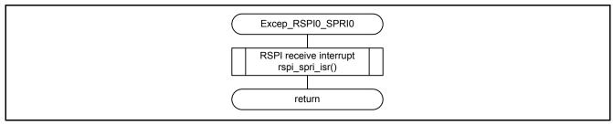
Figure 7.18 RSPI0.SPRI0 Interrupt Handling
