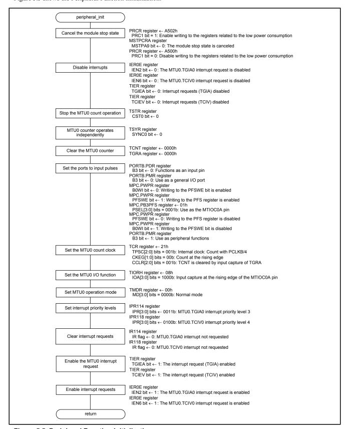
Figure 5.5 Peripheral Function Initialization
