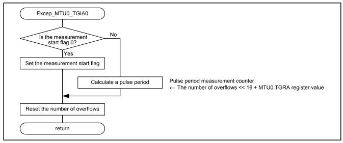
Figure 5.7 MTU0 Input Capture A Interrupt Handler
