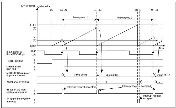
Figure 5.1 Timing Diagram of the Pulse Period Measurement
