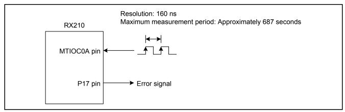
Figure 1.1 Connection Diagram
