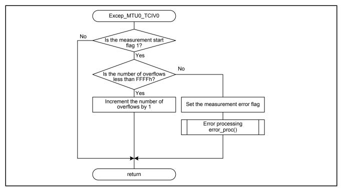
Figure 5.8 MTU0 Overflow Interrupt Handler
