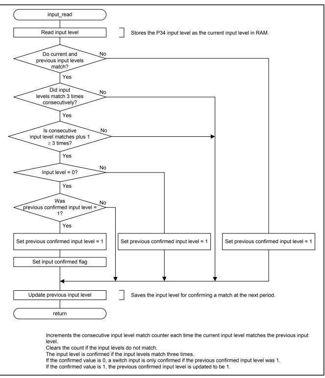
Figure 5.9 Reading Switch Input
