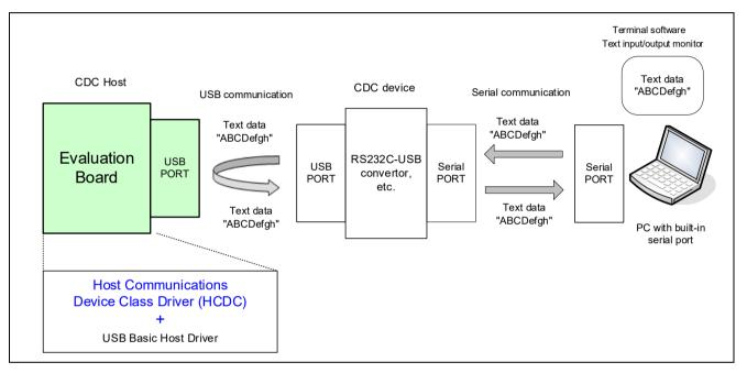
Figure 4-1 Data Transfer (Loopback) Image
