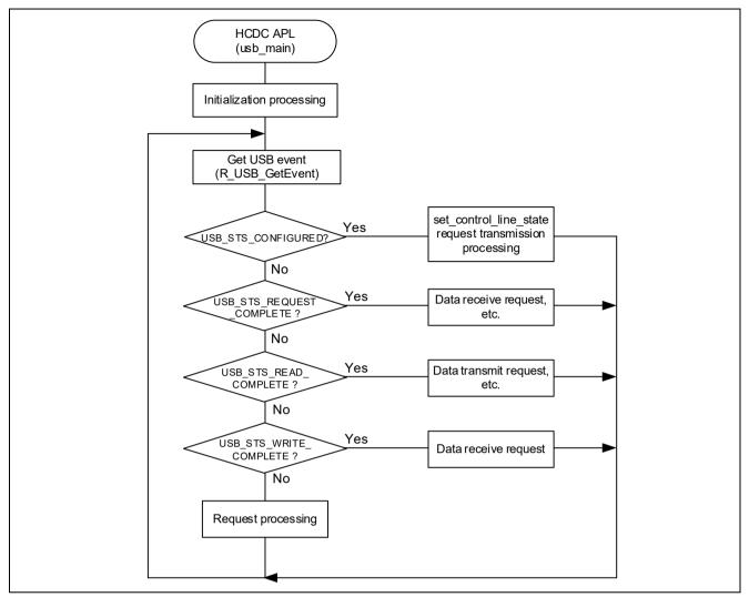
Figure 4-2 Main Loop processing (for Non-OS)
