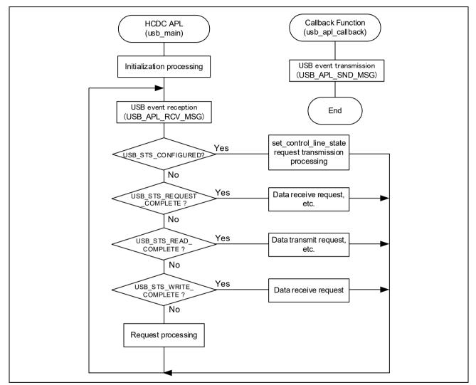
Figure 4-3 Main Loop processing (for RTOS)
