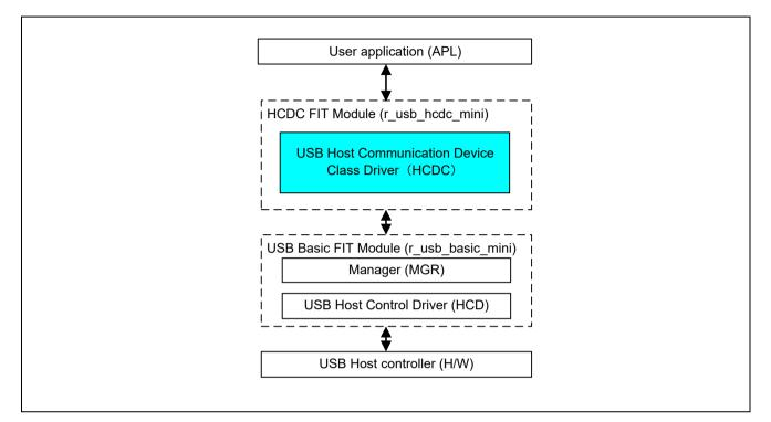
Figure 2-1 Module Configuration
