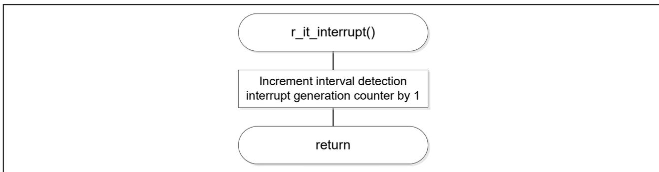
Figure 5.76 12-bit Interval Timer Interrupt Servicing
