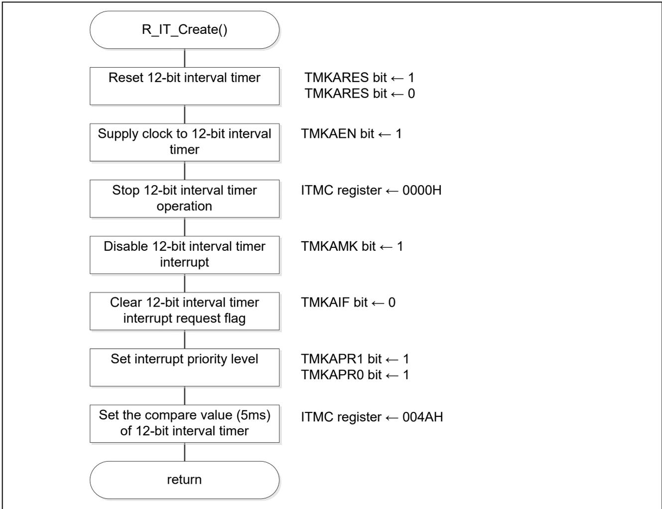
Figure 5.11 12-bit Interval Timer Setting
