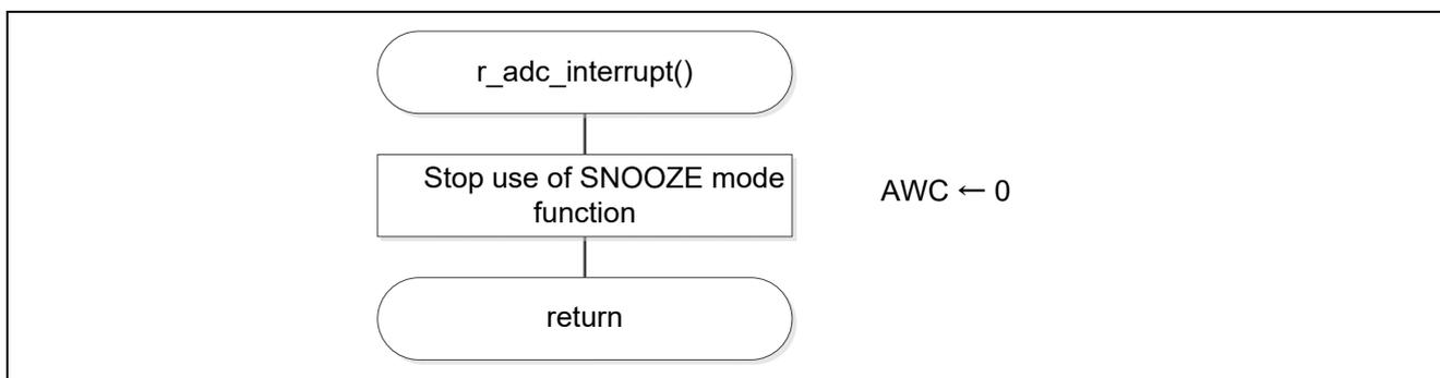
Figure 5.77 A/D Conversion Completion Interrupt Servicing
