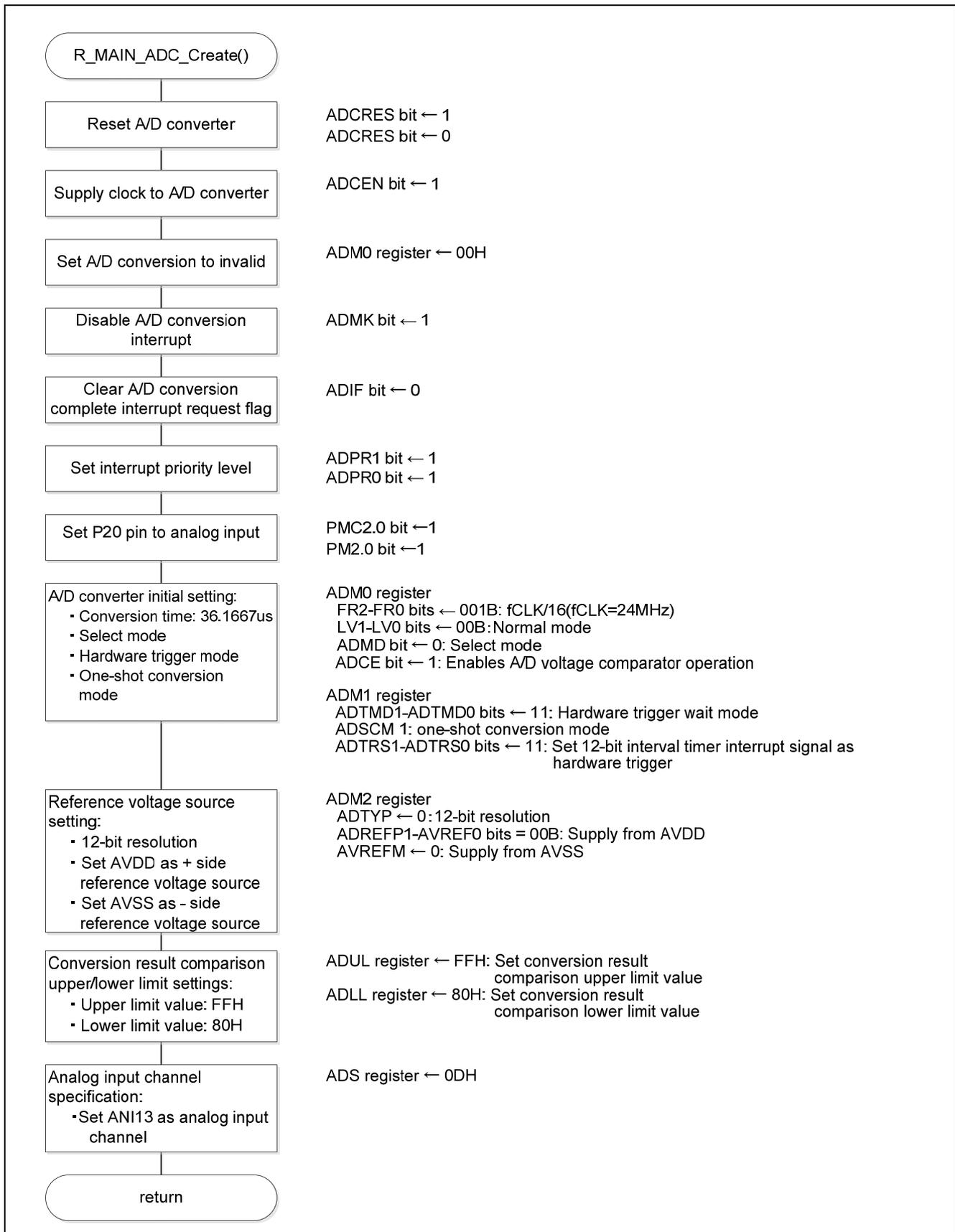
Figure 5.29 A/D Converter Initial Setting
