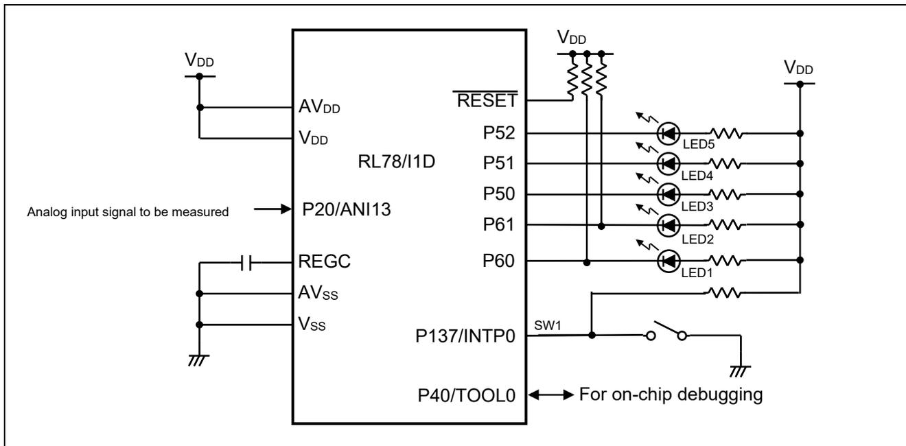
**Figure 4.1 Hardware Configuration**
