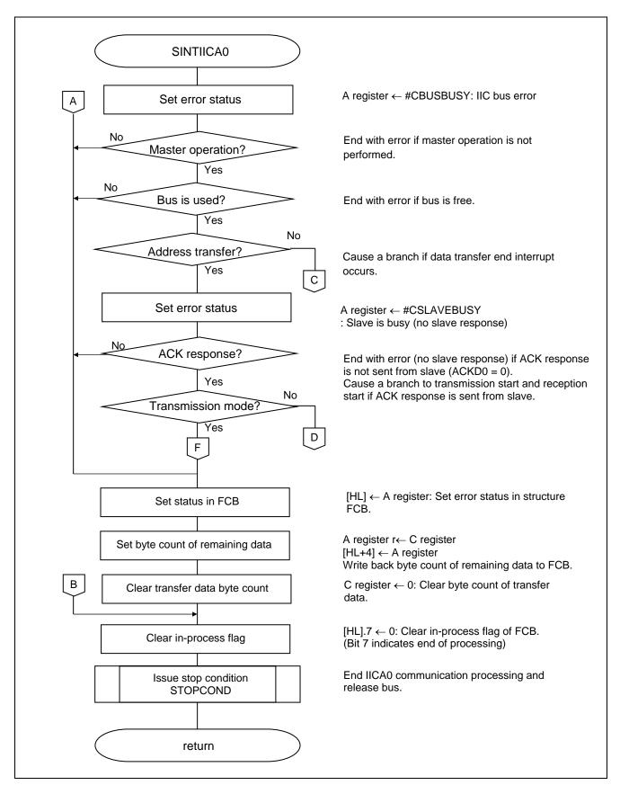
Figure 5.15 IICA0 Master Communication Processing (1/3)
