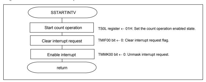
Figure 5.9 Startup of 10-ms interval timer
