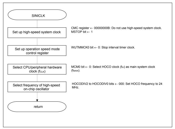
Figure 5.4 Clock Generation Circuit Setup
