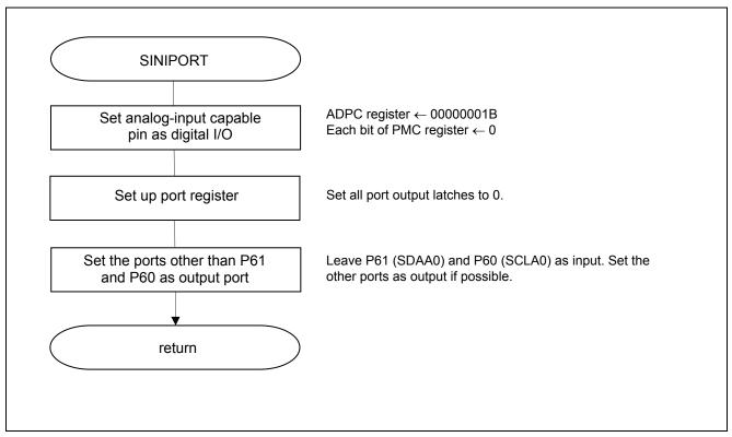
Figure 5.3 I/O Port Setup
