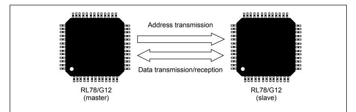
Address transmission: Initial action of the master in IIC communication. This action is intended to identify which slave to transfer data to. After generating a start condition, the master sends one byte of data consisting of 7 bits (indicating the address) and 1 bit (indicating the transfer direction).
