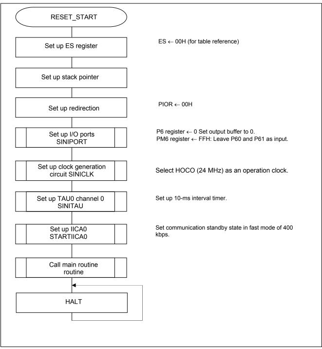
Figure 5.2 CPU Initialization Function
