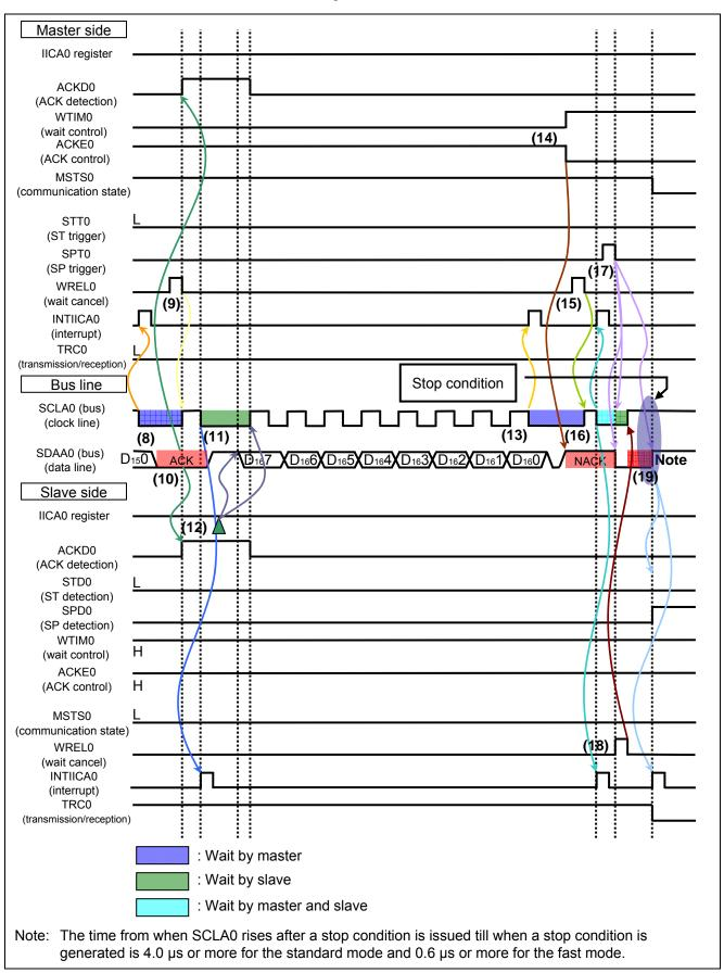
Figure 1.8 IIC Communication Timing Chart (Slave-to-Master Communication Example) (3/3)
