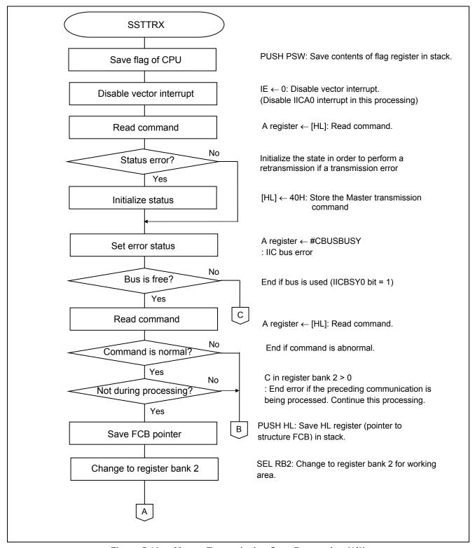
Figure 5.10 Master Transmission Start Processing (1/2)
