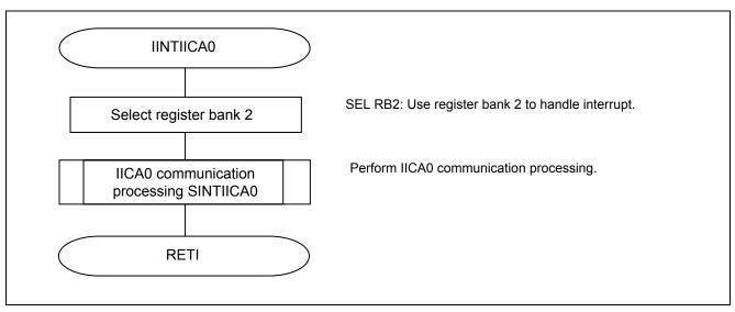
Figure 5.14 IICA0 Interrupt Processing
