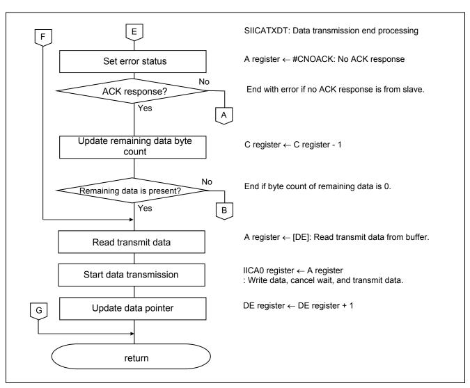
Figure 5.17 IICA0 Master Communication Processing (3/3)
