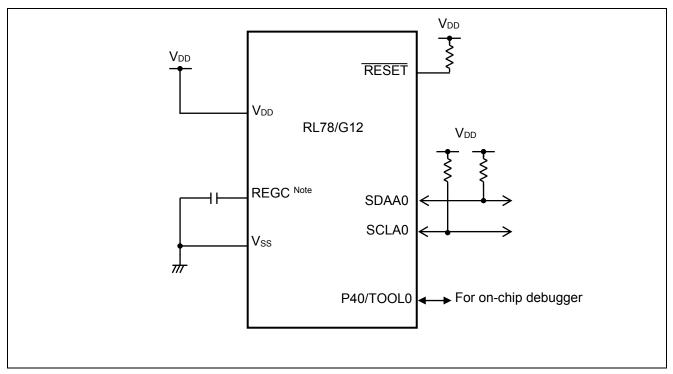
Figure 4.1 Hardware Configuration
