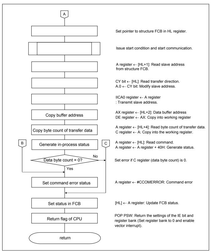
Figure 5.11 Master Transmission Start Processing (2/2)
