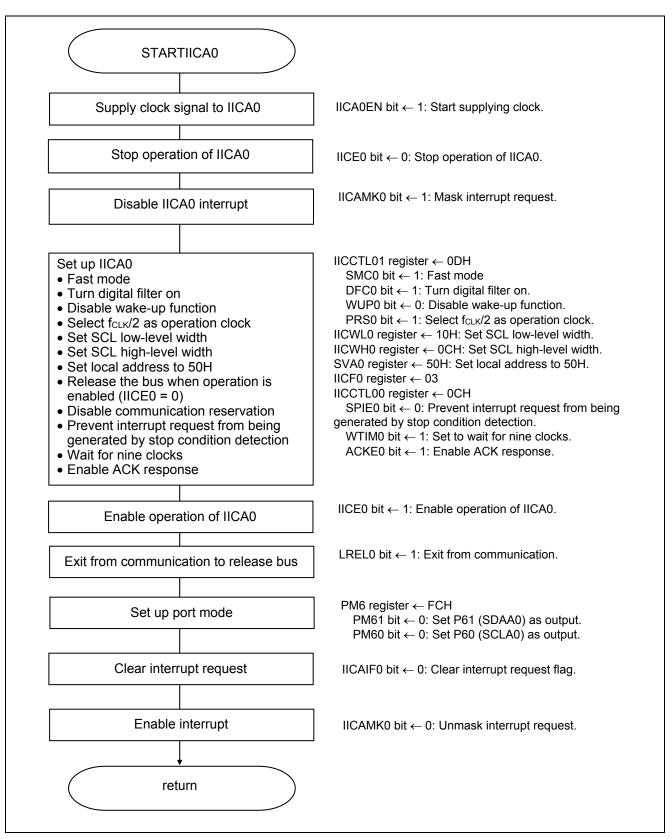
Figure 5.6 Serial Interface IICA Setup
