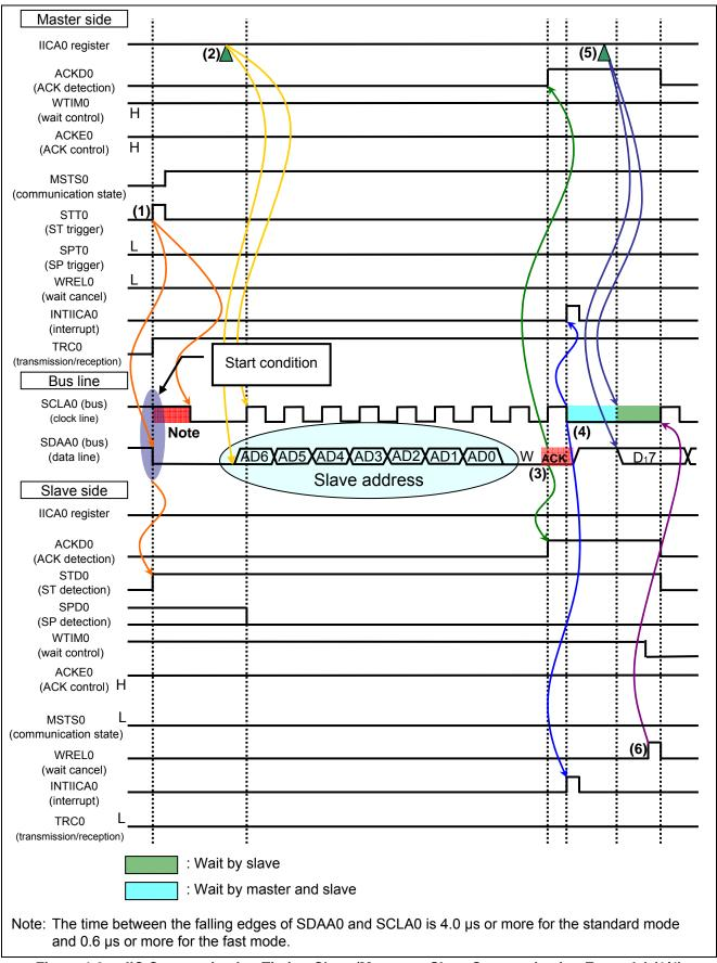
Figure 1.2 IIC Communication Timing Chart (Master-to-Slave Communication Example) (1/4)
