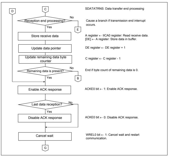
Figure 5.16 IICA0 Master Communication Processing (2/3)
