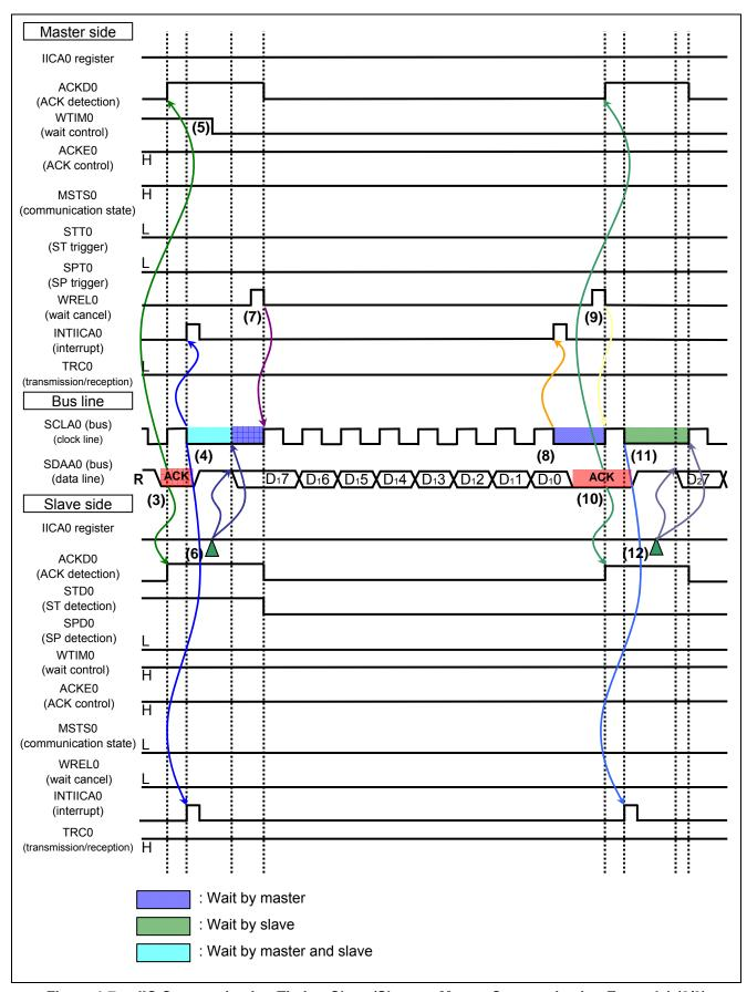
Figure 1.7 IIC Communication Timing Chart (Slave-to-Master Communication Example) (2/3)
