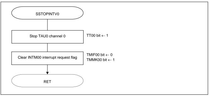
Figure 5.15 Stopping the TAU0 Channel 0
