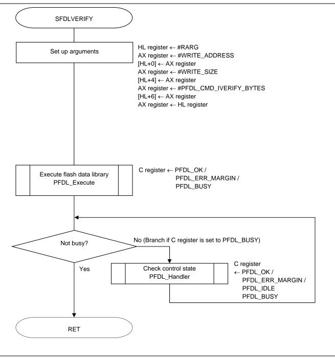
Figure 5.25 Processing the Verify Command
