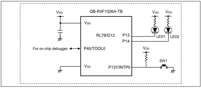
Figure 4.1 Hardware Configuration
