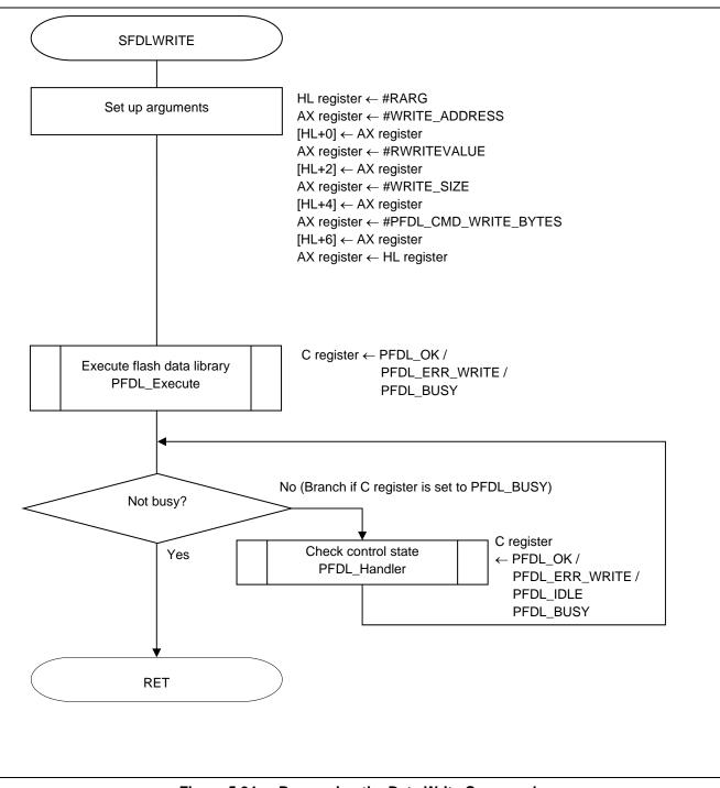
Figure 5.24 Processing the Data Write Command
