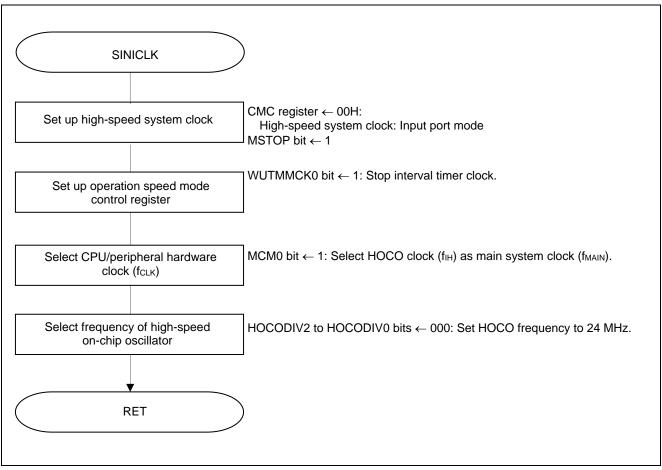
Figure 5.4 Clock Generator Circuit Setup
