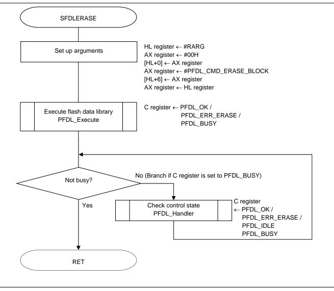
Figure 5.23 Processing the Block Erase Command
