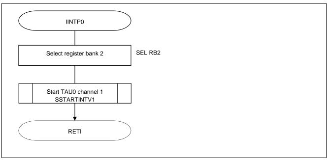
Figure 5.16 Processing the INTP0 External Interrupt
