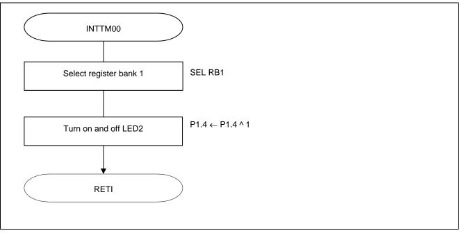
Figure 5.14 Processing the TAU0 Channel 0 Interrupt
