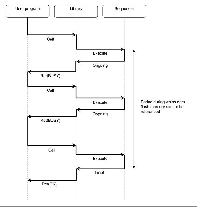
Figure 1.2 Reprogramming Control Example of Data Flash Memory
