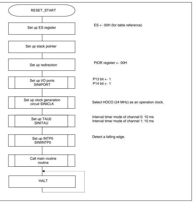
Figure 5.2 CPU Initialization Function
