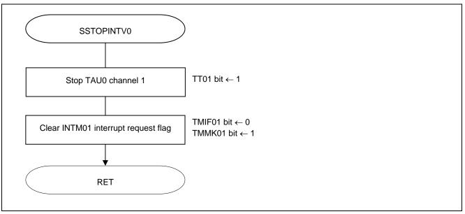
Figure 5.19 Stopping the TAU0 Channel 1
