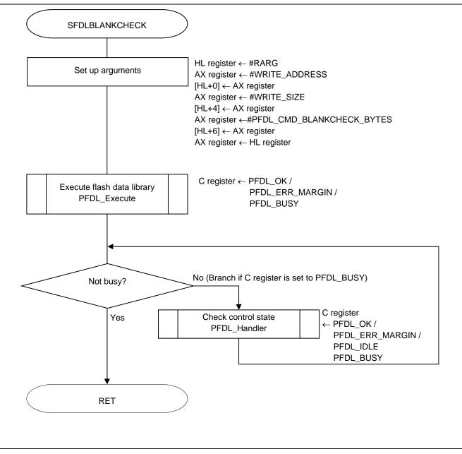
Figure 5.22 Processing the Blank Check Command
