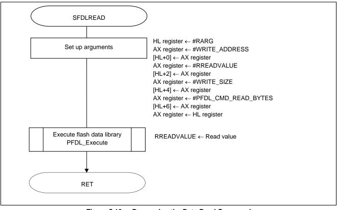
Figure 5.12 Processing the Data Read Command
