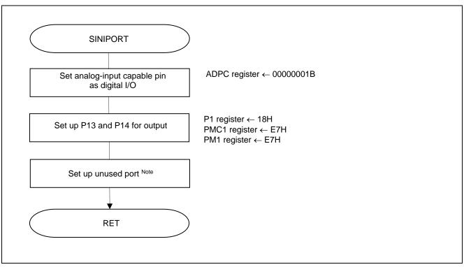
Figure 5.3 I/O Port Setup
