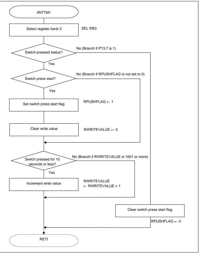
Figure 5.18 Processing the TAU0 Channel 1 Interrupt
