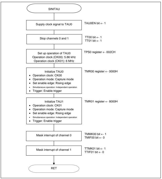
Figure 5.5 Setting up the Timer Array Unit
