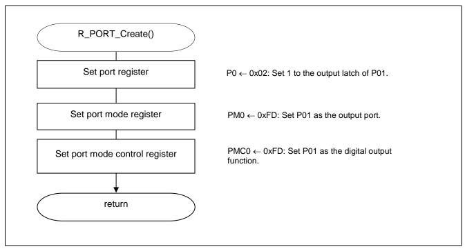
Figure 5.4 I/O Port Setup
