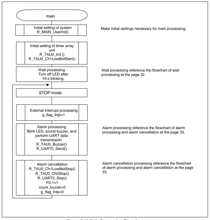
Figure 5.12 Main Processing Flowchart
