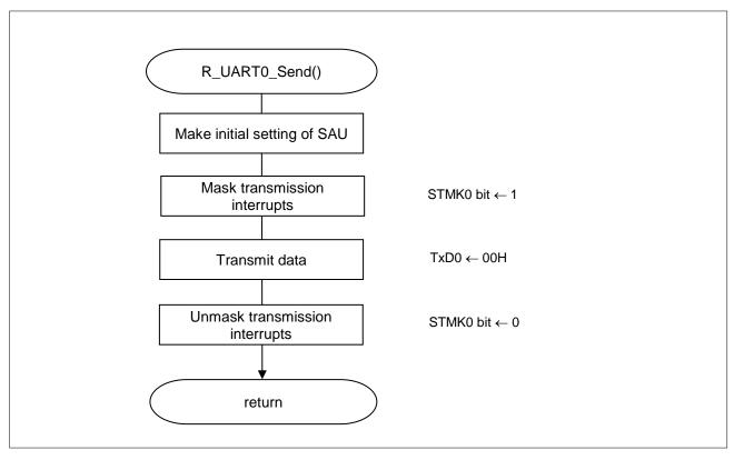
Figure 5.16 Flowchart of UART Data Transmission Function
