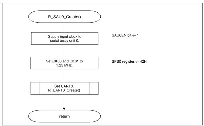
Figure 5.8 Serial Array Unit Setup
