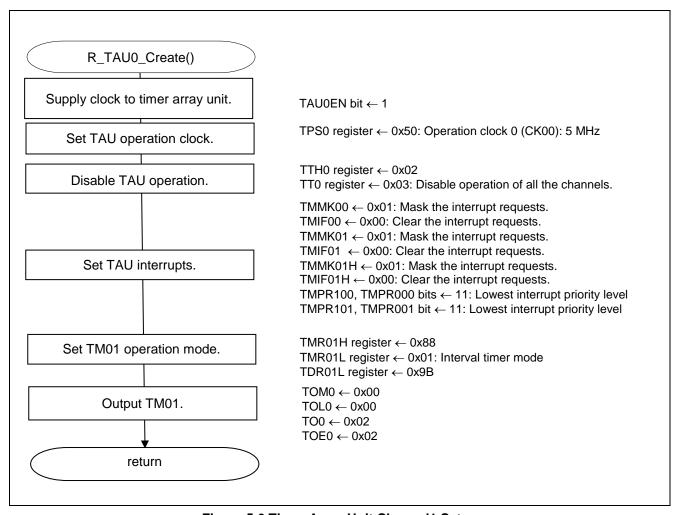
Figure 5.6 Timer Array Unit Channel1 Setup
