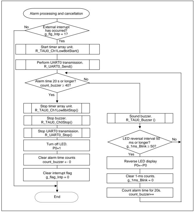
Figure 5.14 Flowchart for Processing and Cancelling Alarm in Main Processing
