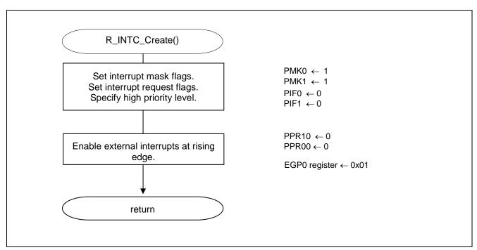
Figure 5.11 External Interrupt Setup
