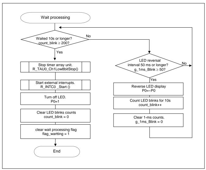
Figure 5.13 Flowchart of Wait Processing in Main Processing
