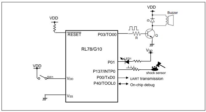
Figure 4.1 the hardware configuration used for this application
