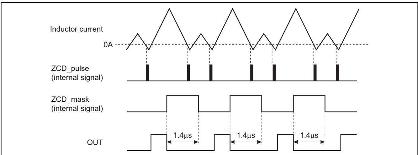
Figure 6 Example of Off Time Control
