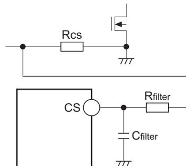
Note: When Rcs becomes smaller, the voltage that is impressed to the terminal of CS becomes smaller. And then, it becomes easy for the restart operation to start at a high input voltage, and it causes the "sound bark", the audio noise of the inductor. This should be noted, when small value of Rcs is utilized to improve efficiency.
