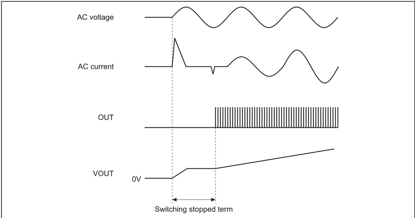
**Figure 7 Example(1) Stop of the Switching Operation**
