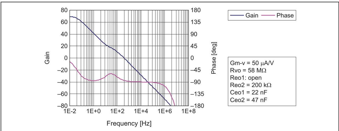
Figure 11 Frequency Characteristics of the Error Amplifier
