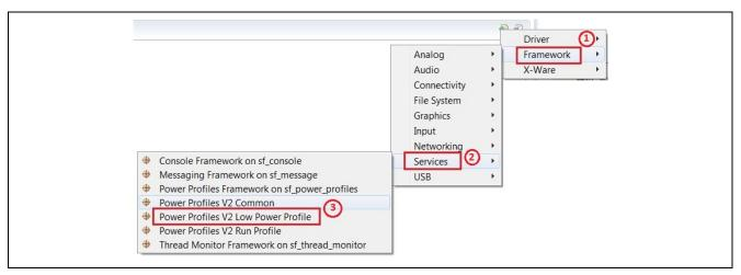
Figure 14 Adding a PPv2 Low Power Profile module
