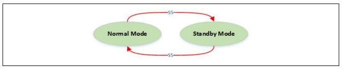
Figure 32 Press the button S5 for selecting a LPM mode
