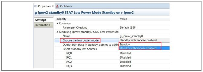
Figure 25 Create a Snooze mode in the Software Standby mode
