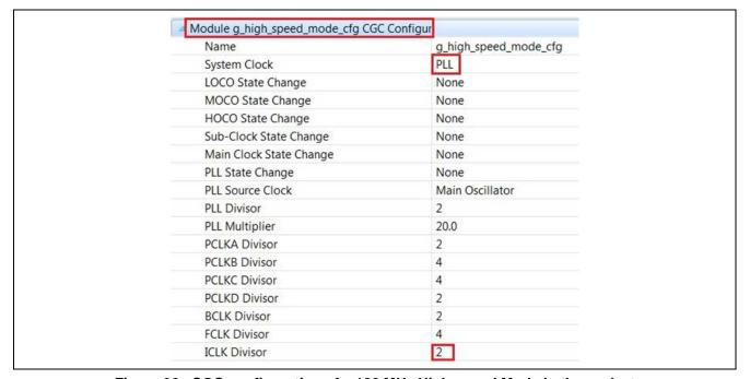
Figure 36 CGC configuration of a 120 MHz High-speed Mode in the project
