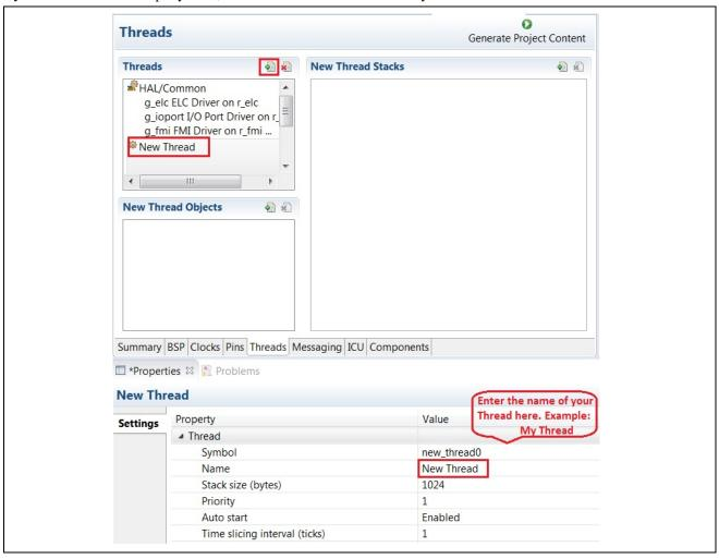
Figure 9 Adding a new thread on the Thread tab
