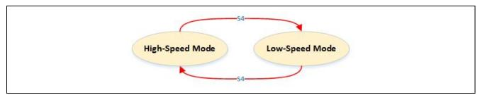
Figure 31 Press the button S4 for selecting a power control mode
