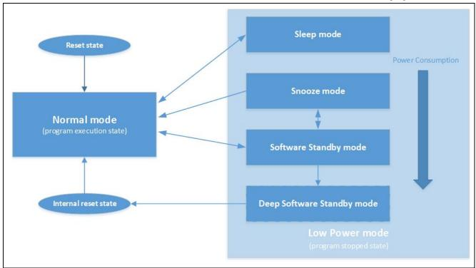
Figure 4 Transitions between the Normal mode and 4 LPM modes
