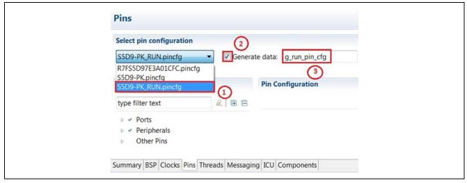
Figure 19 Select a new pin configuration file to be assigned
