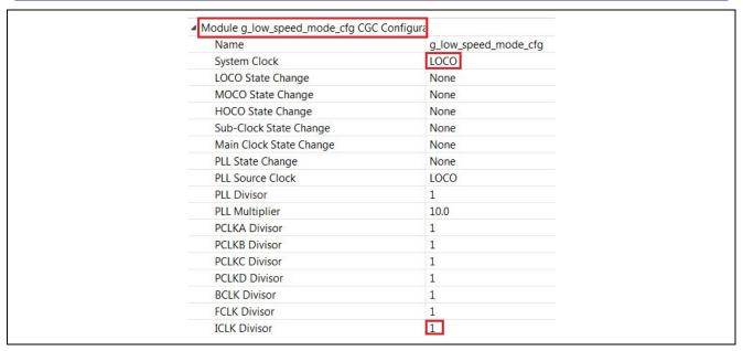
Figure 37 CGC configuration of a 32 kHz Low-speed Mode in the project
