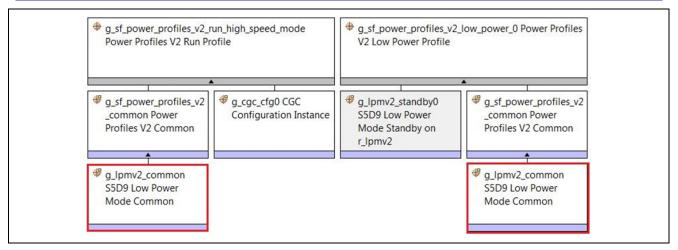
Figure 29 LPM Common module of PPv2 Run/Low Power Profile modules
