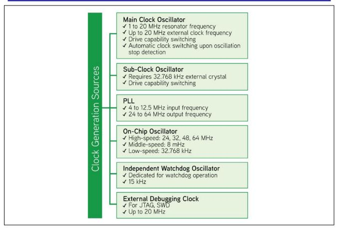
Figure 1 Clock Generation source for Synergy MCU S3 Series
