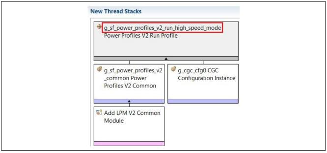
Figure 12 A power control mode defined in the PPv2 Run profile
