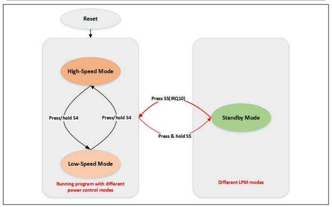
Figure 33 State transitions in the PPv2 project with PK-S5D9
