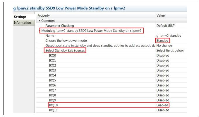
Figure 41 Configuration of the transition between the Standby and Normal modes
