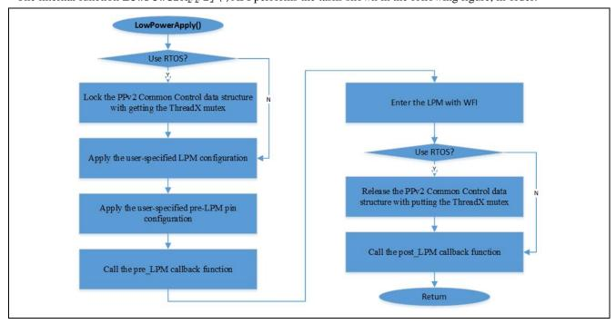
Figure 7 The PPv2 LowPowerApply() process
