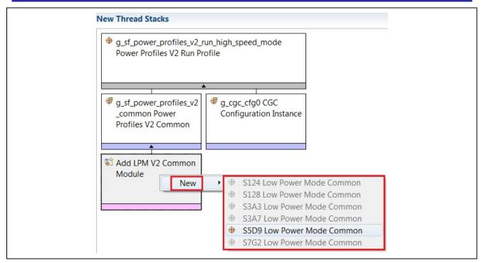
Figure 13 Adding the LPM v2 common module
