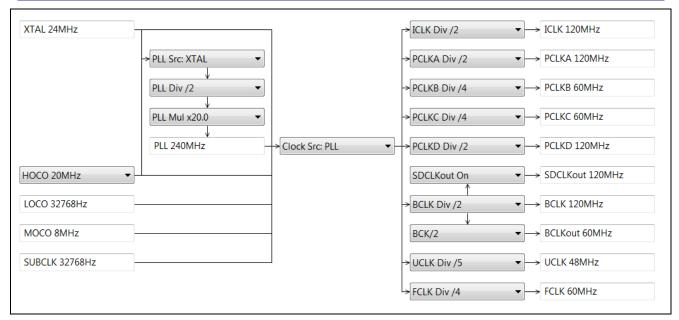
Figure 21 Checking the clock setting for a power control mode
