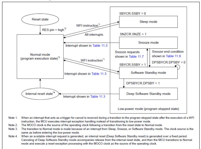
Figure 30 LPM mode transitions for the S5D9 Synergy MCU Group
