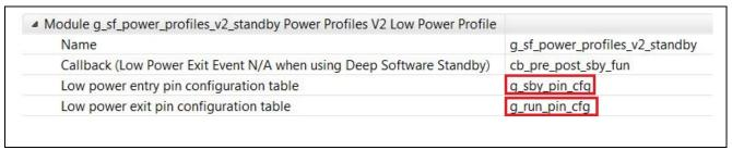
Figure 39 Two pin configuration tables used in the PPv2 application project
