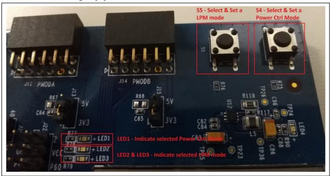
Figure 42 Demonstration setup on the PK-S5D9
