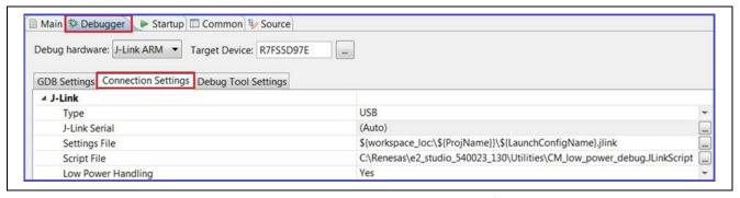
Figure 8 Enabling Low Power Handling in Synergy e<sup>2</sup> studio Debugger
