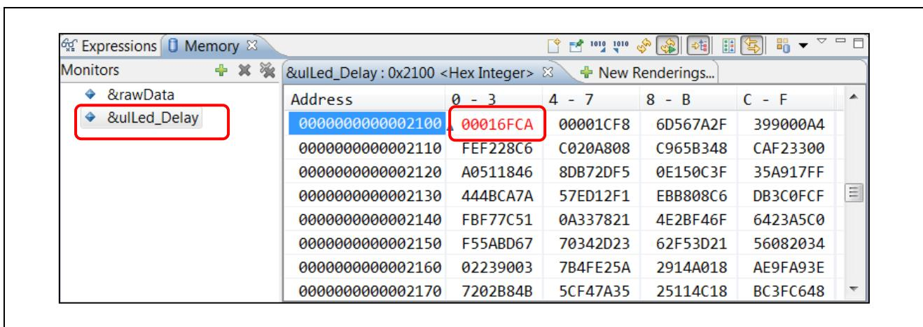
**Figure 9 Memory Rendering Pane – ‘Real-time Refresh’ (when Program is running)**
