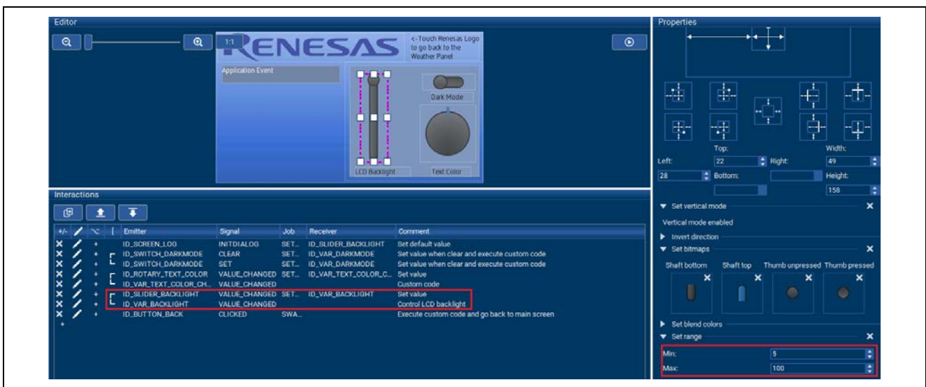
Figure 45. Slider Setup to Control LCD Backlight Intensity
