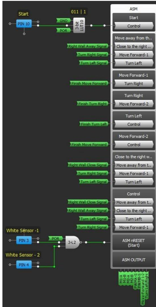
Figure 16: ASM Inputs and Outputs
