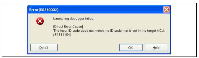
Figure 1.16 The Input ID Code Does Not Match the ID Code That is Set in the Target MCU
