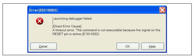
Figure 1.15 The Signal on the RESET Pin is Active
