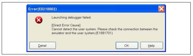
Figure 1.7 Cannot Detect the User System
