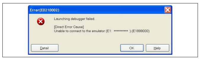
Figure 1.8 Unable to Connect to the Emulator
