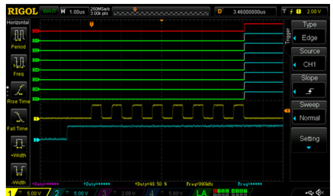
Figure 6. 1us scale of Data Byte 0xFF
