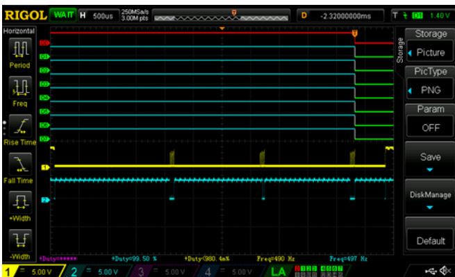
Figure 3. I2C Command [0x00, 0xF4, 0x00]
