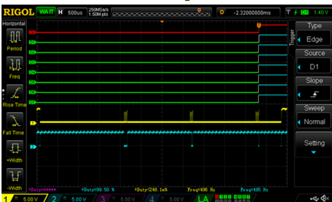
Figure 4. I2C Command [0x00, 0xF4, 0xFF]
