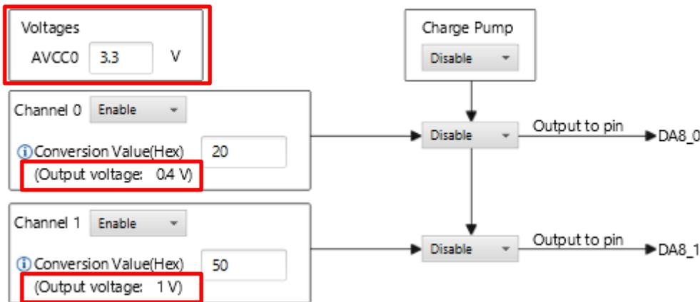
Figure 1-3. AVCC0 and DAC output voltage value
