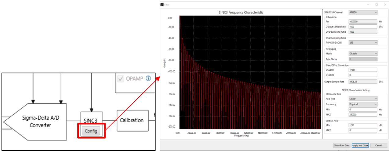
Figure 1-2. SINC3 filter setting
