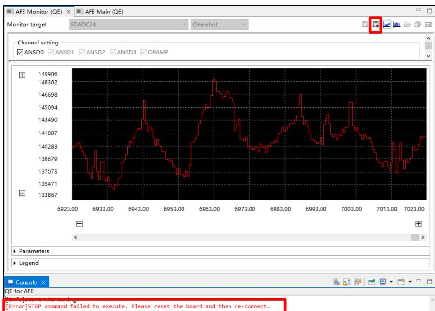
Figure 3-4 Stop Failed Case
