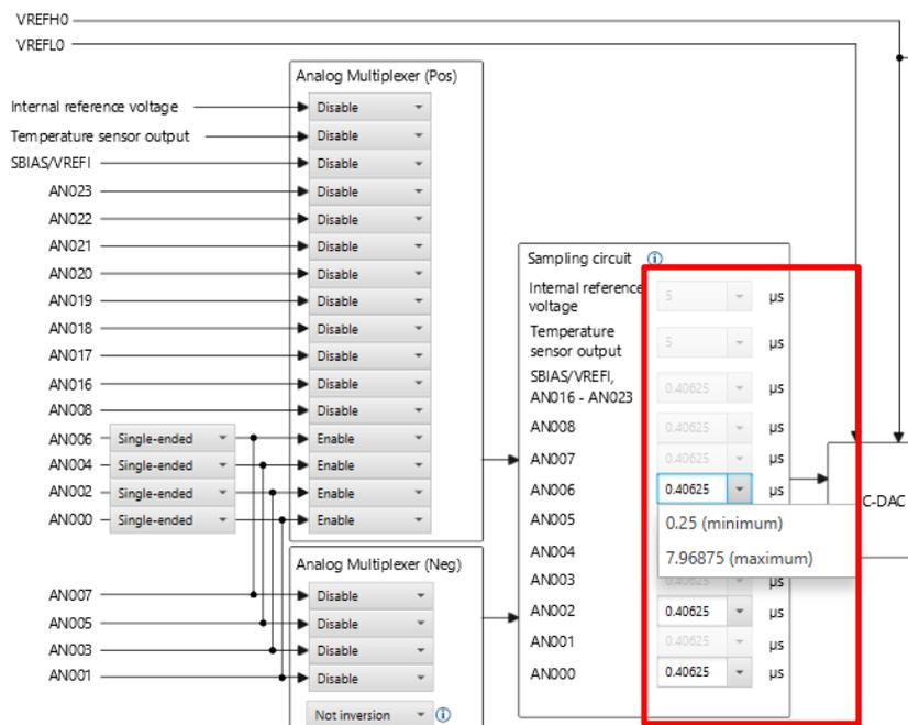
Figure 1-1. ADC16 sampling time selection
