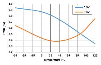
Figure 18. 5.5V Pulse-Width Distortion vs Temperature vs V<sub>DD</sub> Voltage
