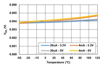
Figure 20. Logic Low Output Voltage vs Temperature
