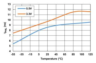
Figure 14. Propagation Delay (High-to-Low) vs Temperature vs V<sub>DD</sub> Voltage
