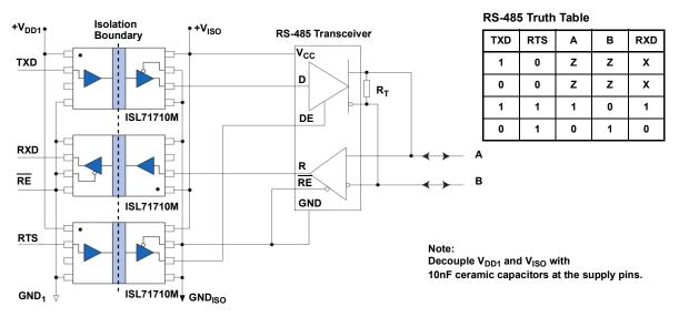
Figure 3. RS-485 Multi-Chip Isolated Transceiver Application Schematic
