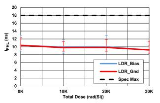
Figure 30. 5.5V Propagation Delay (High-to-Low) vs TID
