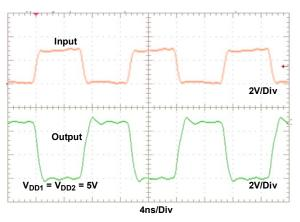
Figure 10. 75MHz Input and Output Waveforms
