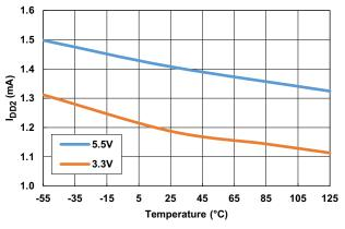
Figure 13. Output Quiescent Supply Current vs Temperature vs V<sub>DD2</sub> Voltage
