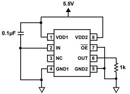
Figure 33. 5.5V Logic Input Current - High vs TID
