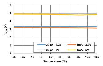
Figure 21. Logic High Output Voltage vs Temperature
