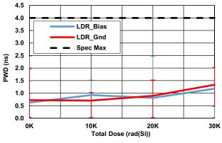
Figure 31. 5.5V Pulse-Width Distortion vs TID
