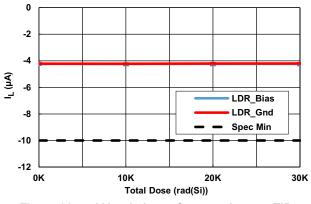
Figure 32. 5.5V Logic Input Current - Low vs TID
