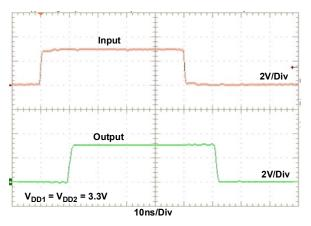
Figure 2. 10MHz Input and Output Waveforms
