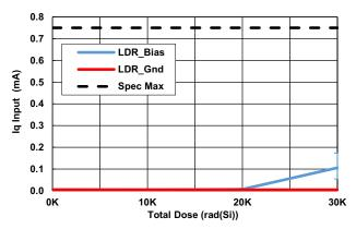
Figure 28. 5.5V Input Quiescent Supply Current vs TID
