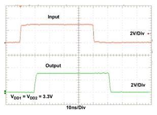
Figure 6. 10MHz Input and Output Waveforms
