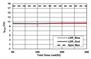
Figure 29. 5.5V Propagation Delay (Low-to-High) vs TID
