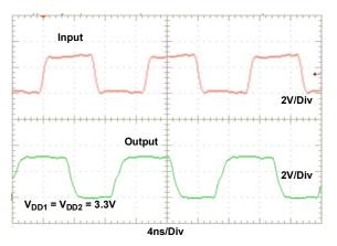
Figure 8. 75MHz Input and Output Waveforms
