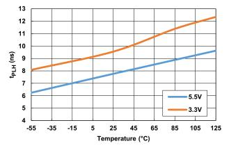
Figure 15. Propagation Delay (Low-to-High) vs Temperature vs V<sub>DD</sub> Voltage
