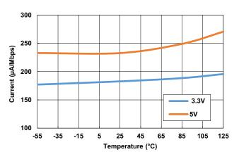
Figure 19. Dynamic Power Consumption vs Temperature
