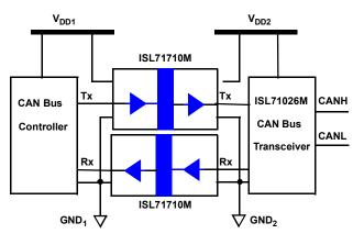
Figure 1. Typical CAN Bus Application
