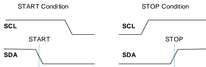
Figure 5. START and STOP Condition Waveform
