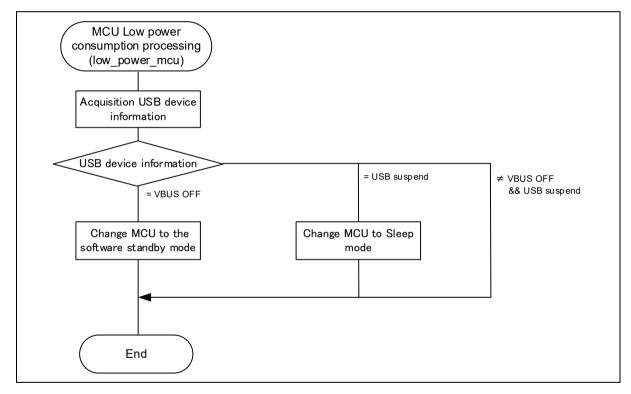
Figure 4-5 Flowchart of MCU Low Power Consumption Processing
