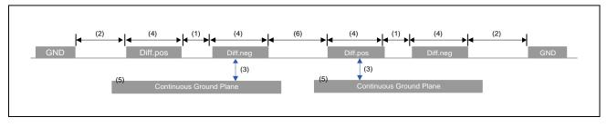
Figure 1.3 Signal Lines Example.2
