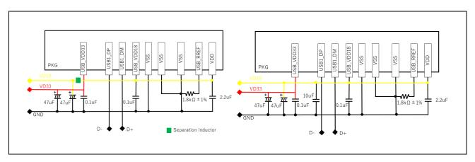
Figure B.1 Configuration of External Parts in the Case of 1 Port (left: with separation inductor, right: without separation inductor)
