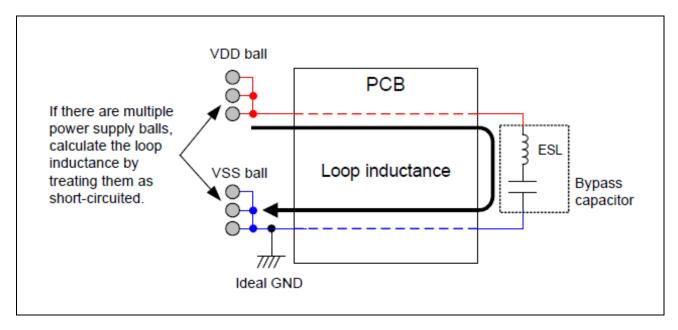
Figure A.1 Concept of Loop Inductance
