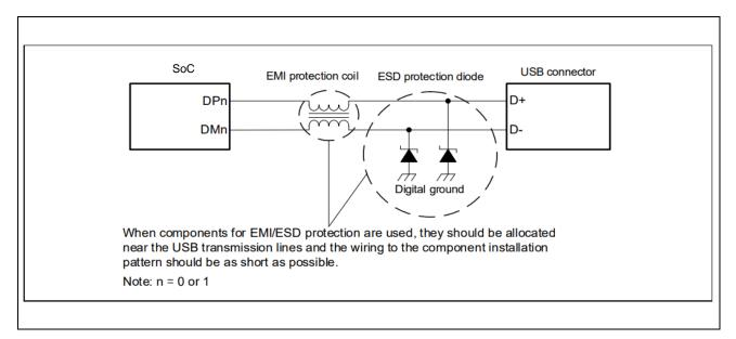
Figure D.1 Connection Example when Components for EMI/ESD Protection are Used
