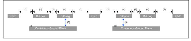
Figure 1.2 Signal Lines Example.1
