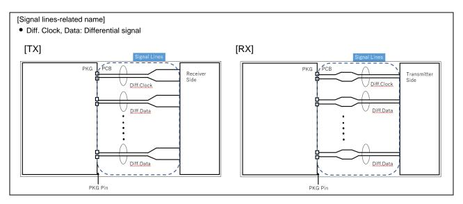
Figure 1.1 Signal Line Topology of MIPI-CSI and MIPI-DSI
