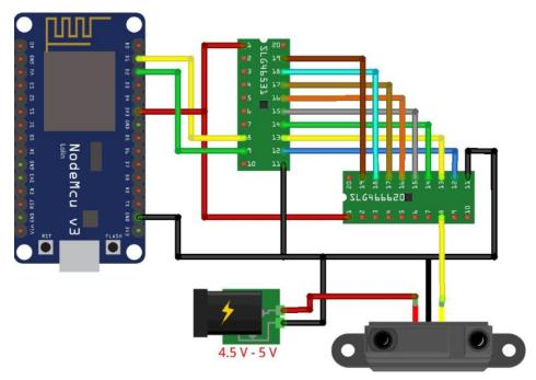
Figure 20: Hardware Connections
