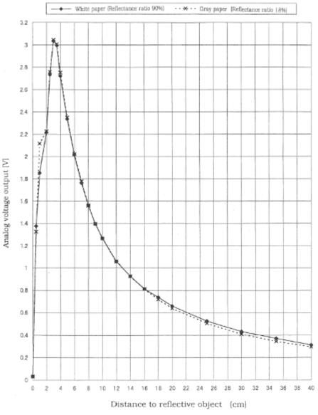
Figure 18: Sharp Sensor Distance-voltage Graph
