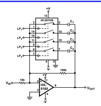
FIGURE 5. LOW PASS FILTER WITH SELECTABLE BREAK FREQUENCY - SWITCH SELECTION PLACES VARIOUS VALUES OF CAPACITANCE IN PARALELL WITH THE FEEDBACK RESISTOR. THE VALUE OF THE CAPACITOR DETERMINES THE BREAK FREQUENCY. THE BREAK FREQUENCY IS THAT FREQUENCY AT WHICH THE SIGNAL BEGINS ATTENUATION
