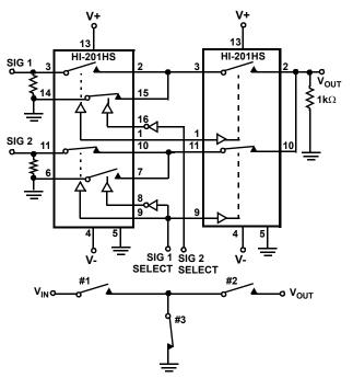
FIGURE 8. VIDEO SWITCHING WITH IMPROVED ISOLATION -IMPROVED HIGH FREQUENCY OFF STATE PERFORMANCE IS OBTAINED BY USING A T-SWITCH CONFIGURATION. WHEN TWO SERIES SWITCHES ARE OFF, THE THIRD SWITCH IS SHORTED TO GROUND
