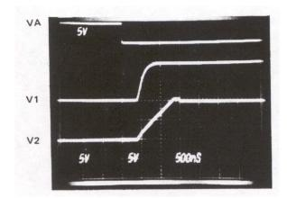
FIGURE 3B. CIRCUIT RESPONSE TO A "SAMPLE" COMMAND USING A STANDARD 201 AND AN HA-5100 OPERATIONAL AMPLIFIER (AQUISITION TIME = 1.5µS)
