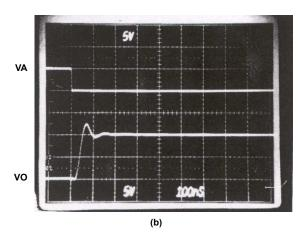
FIGURE 2. HIGH SPEED ANALOG MULTIPLEXER: (a) CIRCUIT RESPONSE USING THE STANDARD 201 ( $t_{access} = 400$ ns). (b) CIRCUIT RESPONSE USING HI-201HS ( $t_{access} = 50$ ns). THE ACCESS TIME IS DEFINED AS TOTAL TIME REQUIRED TO ACTIVATE AN "OFF" SWITCH TO THE "ON" STATE. ACCESS TIME IS NORMALLY MEASURED FROM THE INITIATION OF THE DIGITAL INPUT PULSE ( $V_A$ ) TO THE 90% POINT OF THE OUTPUT TRANSITION.
