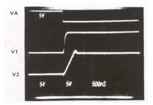
FIGURE 3C. CIRCUIT RESPONSE USING AN HI-201HS AND HA-5160: HI-201HS SIGNIFICANTLY REDUCES SWITCH DELAY TIME (AQUISITION TIME = 500ns)
