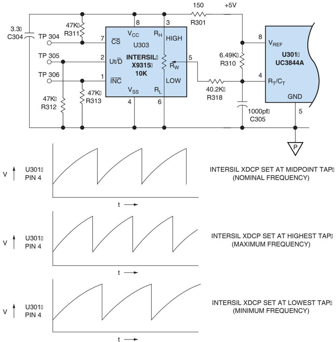
FIGURE 7. XDCP CONVERTOR FREQUENCY CONTROL
