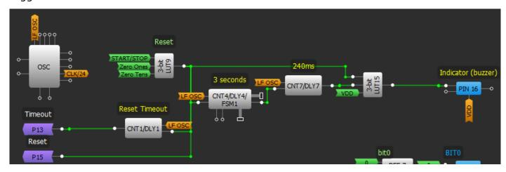
Figure 7. Buzzer and Reset Timeout
