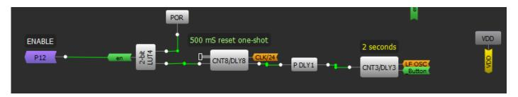
Figure 6. 5 second triggered 500mS Reset One-Shot
