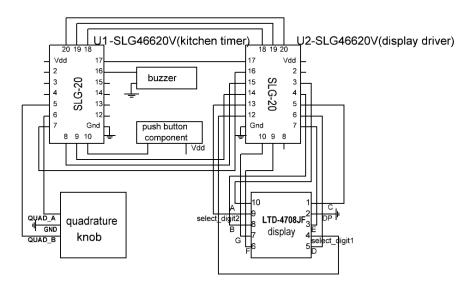
Figure 1. System Level Diagram
