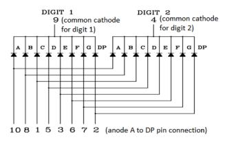
Figure 9. LTD-4708JF Pin Connection
