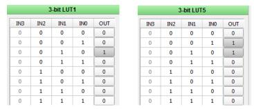
Figure 4. CW (3-bit LUT1) and CW or CCW (3-bit LUT5) Properties
