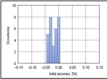
Figure 39.99 Initial Accuracy of Voltage Reference (AVCC0 = 5.0 V, 30 samples)
