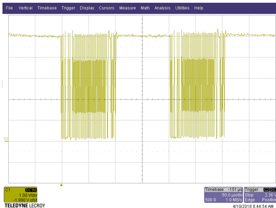
Figure 2. Oscilloscope Plot of Two Data Packets
