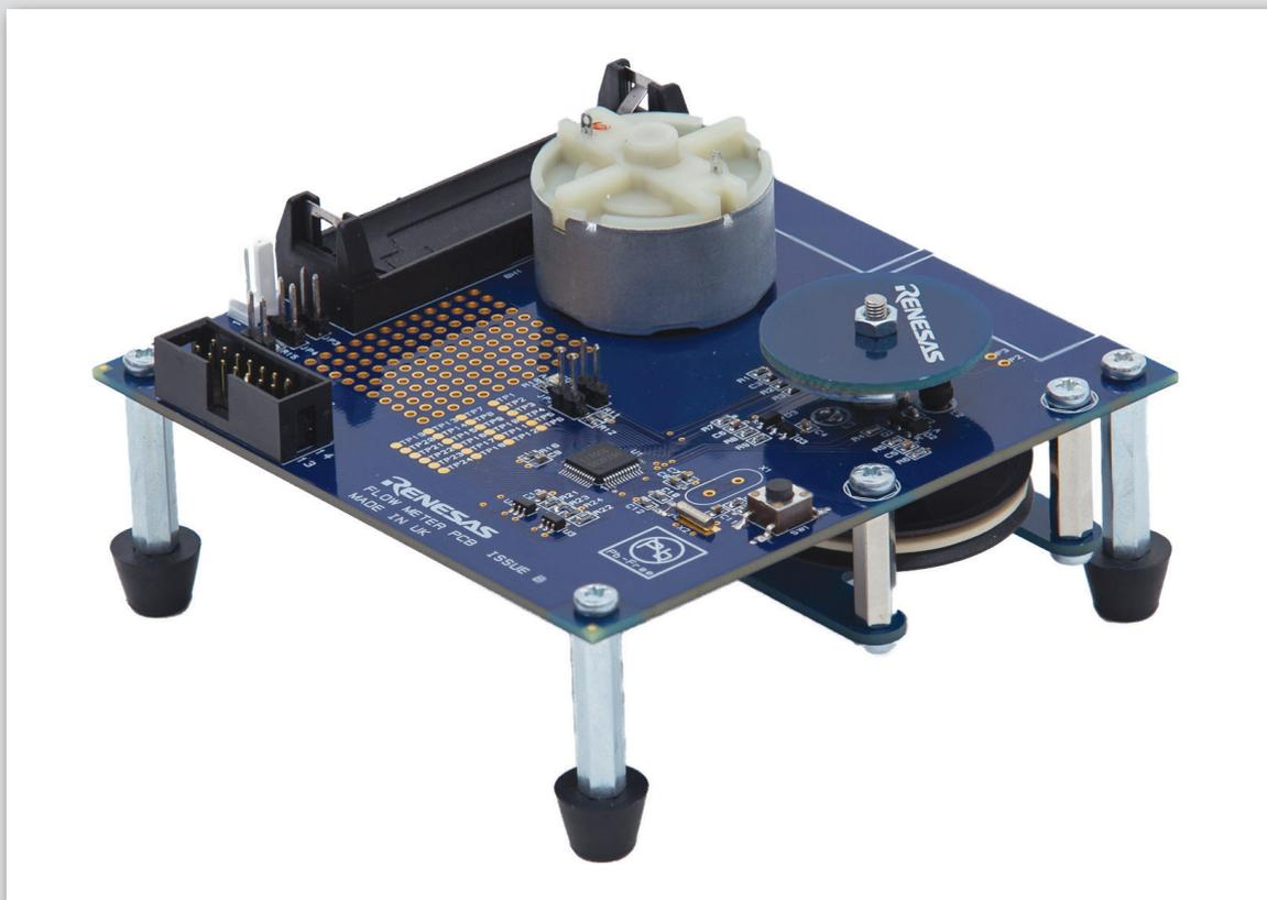
The sensor disk's RPM may be controlled by tuning the motor's DC voltage. An optical sensor is included to determine the exact RPM of the disk.
