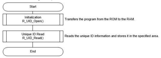
Figure 1.1 Processing Example of the UID FIT Module
