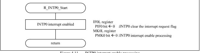
Figure 4.11 INTP0 interrupt enable processing
