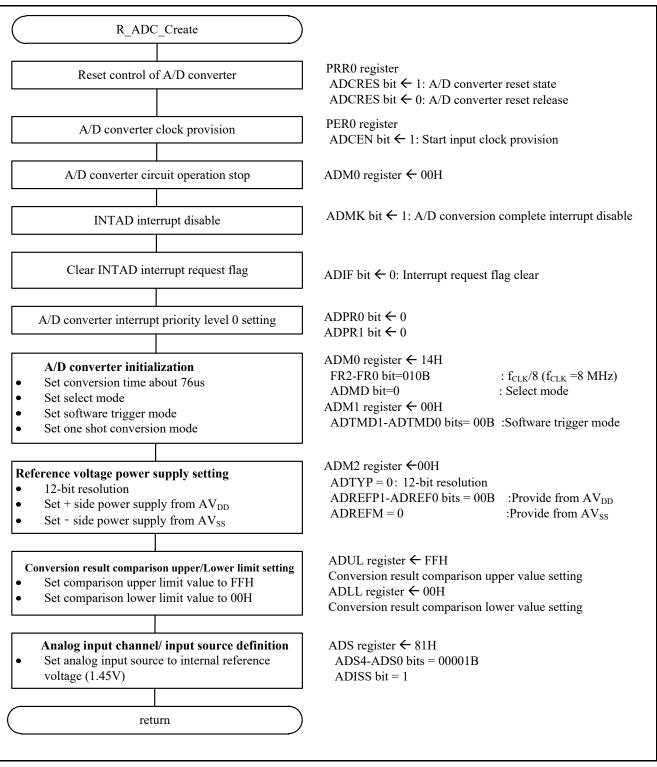
Figure 4.20 A/D converter initialization
