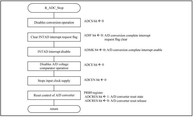
Figure 4.22 A/D converter stop processing
