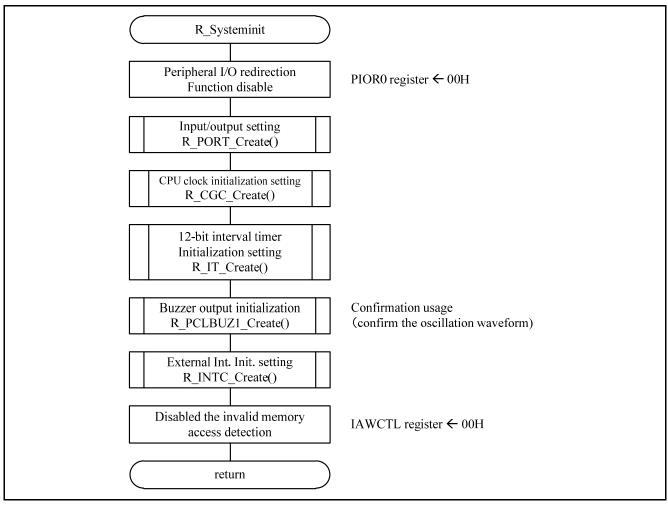
Figure 4.4 Peripheral function initialization
