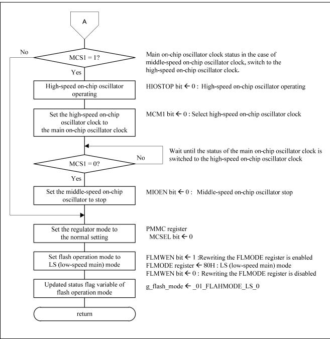
Figure 4.16 Flash operation mode switching (LS normal) processing(2/2)
