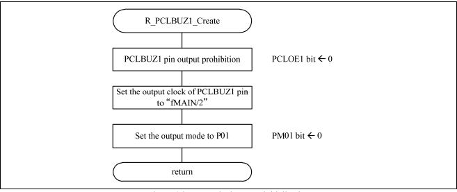
Figure 4.8 clock output initialization
