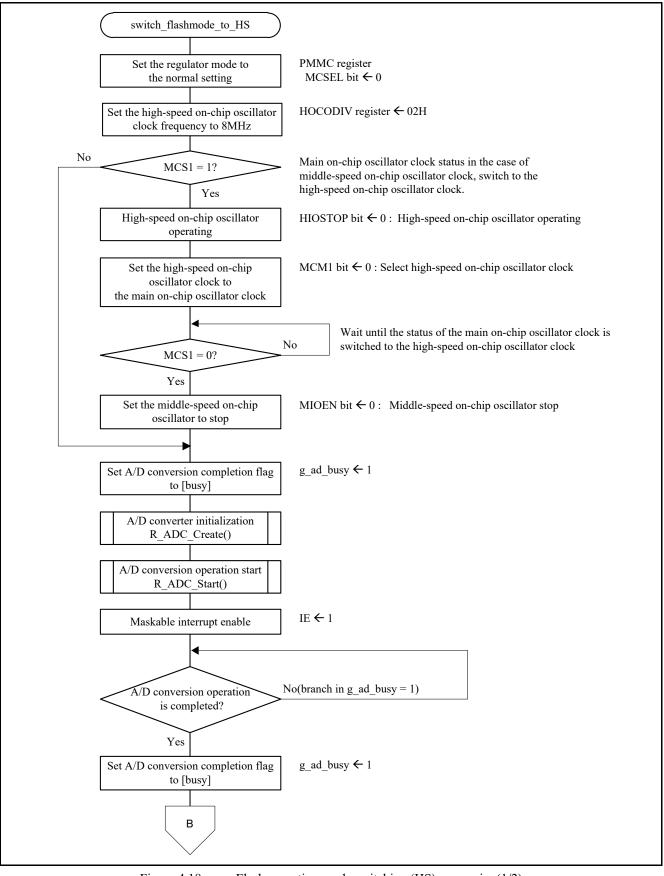
Figure 4.18 Flash operation mode switching (HS) processing(1/2)
