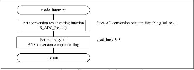
Figure 4.27 A/D conversion complete interrupt processing
