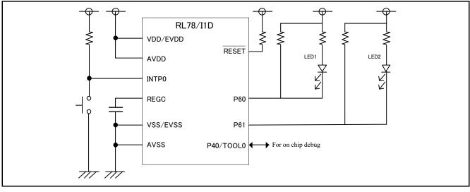
Figure 3.1 Hardware structure
