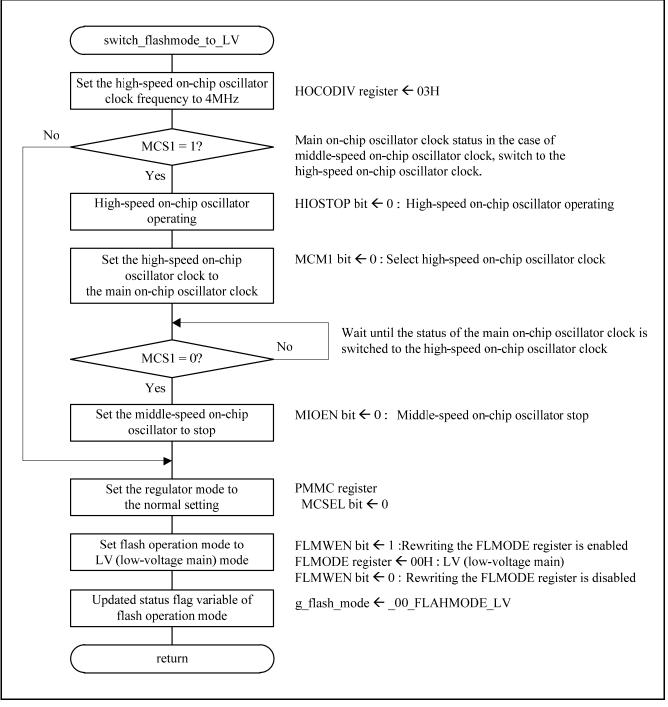
Figure 4.14 Flash operation switching (LV) processing
