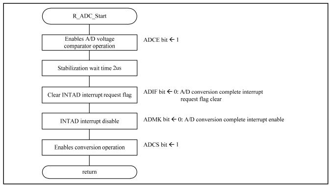
Figure 4.21 A/D conversion operation start processing
