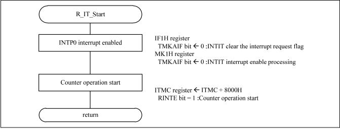
Figure 4.12 12-bit interval timer start processing
