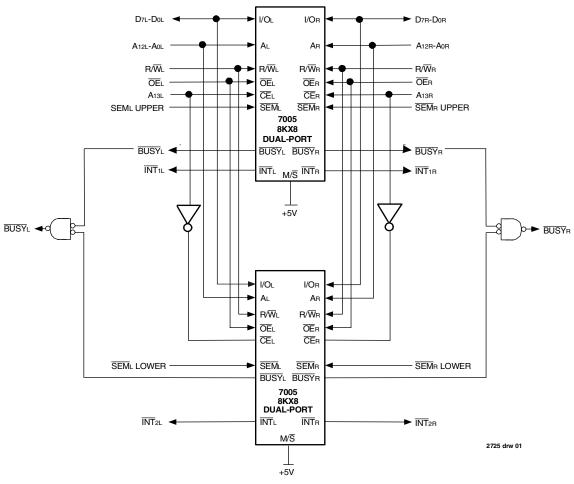
Figure 1. Depth Expansion of the IDT7005 8k x 8 Dual-Port
