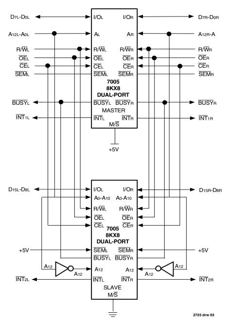
Figure 3. Width Expansion with More Interrupts
