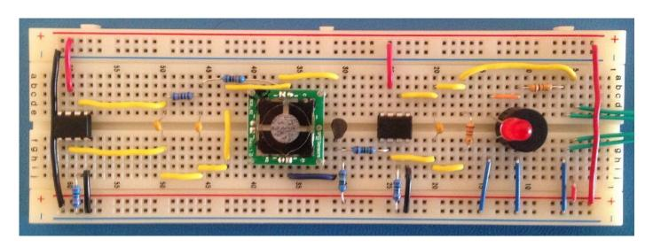
Figure 3. The potentiostat and LED/Alarm circuit prototyped on a breadboard. The protruding green wires connect to the GreenPAK Universal Development Board. For a full list of the external components used, see Appendix
