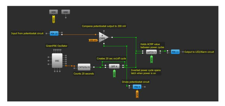
Figure 14. The internal connections of the GreenPAK4 blocks
