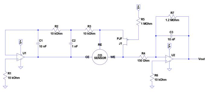
Figure 1. The potentiostat schematic for the SPEC CO sensor 100-102. CE, RE, and WE stand for Counter Electrode, Reference Electrode, and Working Electrode, respectively
