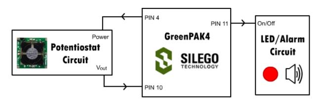
Figure 4. High-level block diagram of the full CO detector system
