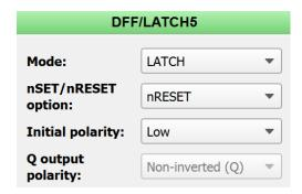
Figure 12. Configuration of the latch used to save the comparator values
