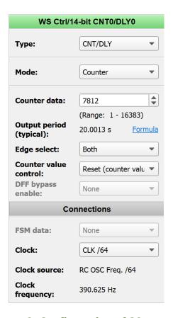
Figure 9. Configuration of 20 second counter
