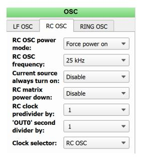
Figure 11. Configuration of the oscillator. Note the power mode has been switched to "Force power on."
