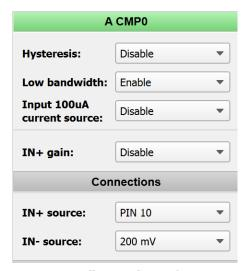
Figure 7. Configuration of ACMP0 with the IN- source (the reference) set to 200 mV. If the IN+ source (PIN 10) exceeds 200 mV, the output will be high; otherwise, the output is low
