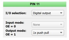
Figure 13. Configuration of PIN 11, which drives the LED/Alarm circuit
