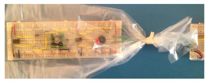
Figure 15. Testing the system by placing the potentiostat and LED/Alarm circuit inside a plastic bag with approximately 400 ppm of CO. The green wires pass through the opening of the bag to connect to the GreenPAK Universal Development Board (not shown)
