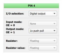
Figure 8. Configuration of PIN 4
