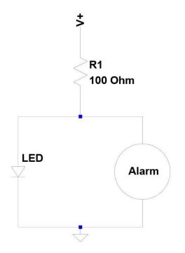
Figure 2. The external circuit to drive the LED and alarm. More information on these components can be found in the Appendix at end
