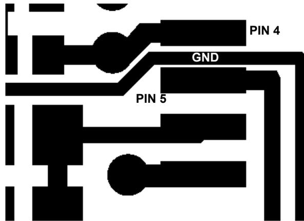
FIGURE 15. LAYOUT DETAIL OF GND BETWEEN PINS 4 AND 5
