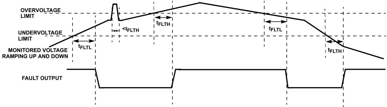
FIGURE 3. ISL8702A, ISL8703A, ISL8704A, ISL8705A FAULT OPERATIONAL DIAGRAM
