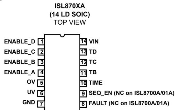
ISL8701A, ISL8703A, ISL8705A PINS 1-4 ARE ENABLE# FUNCTION
