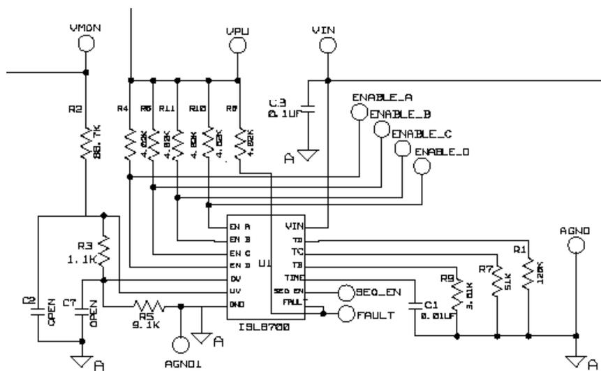
FIGURE 16. ISL8700XAEVAL1 PHOTOGRAPH AND SCHEMATIC OF LEFT CHANNEL
