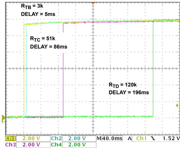
FIGURE 8. ENABLE\_X TO ENABLE\_X ENABLING
