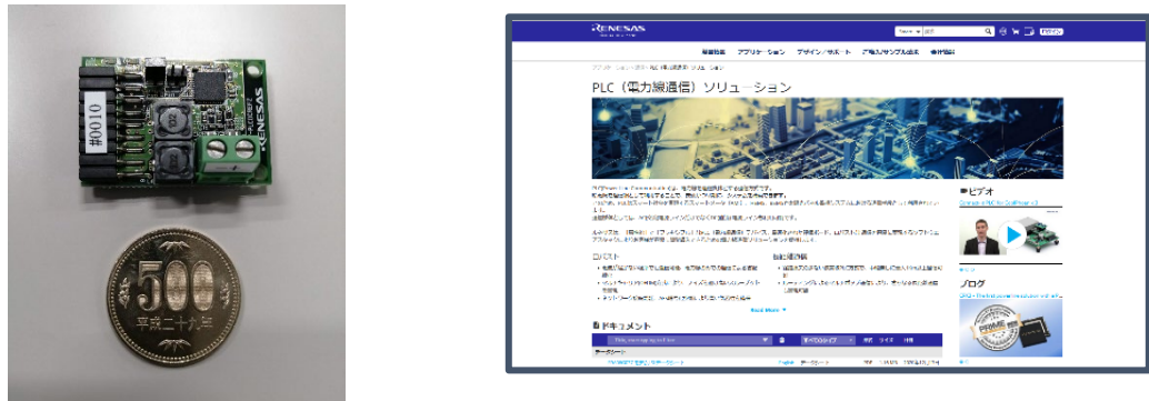
Figure 5. R9A06G061 DC Communication Module (3.8cm x 2.8cm) Documentation Available on the Renesas Website
