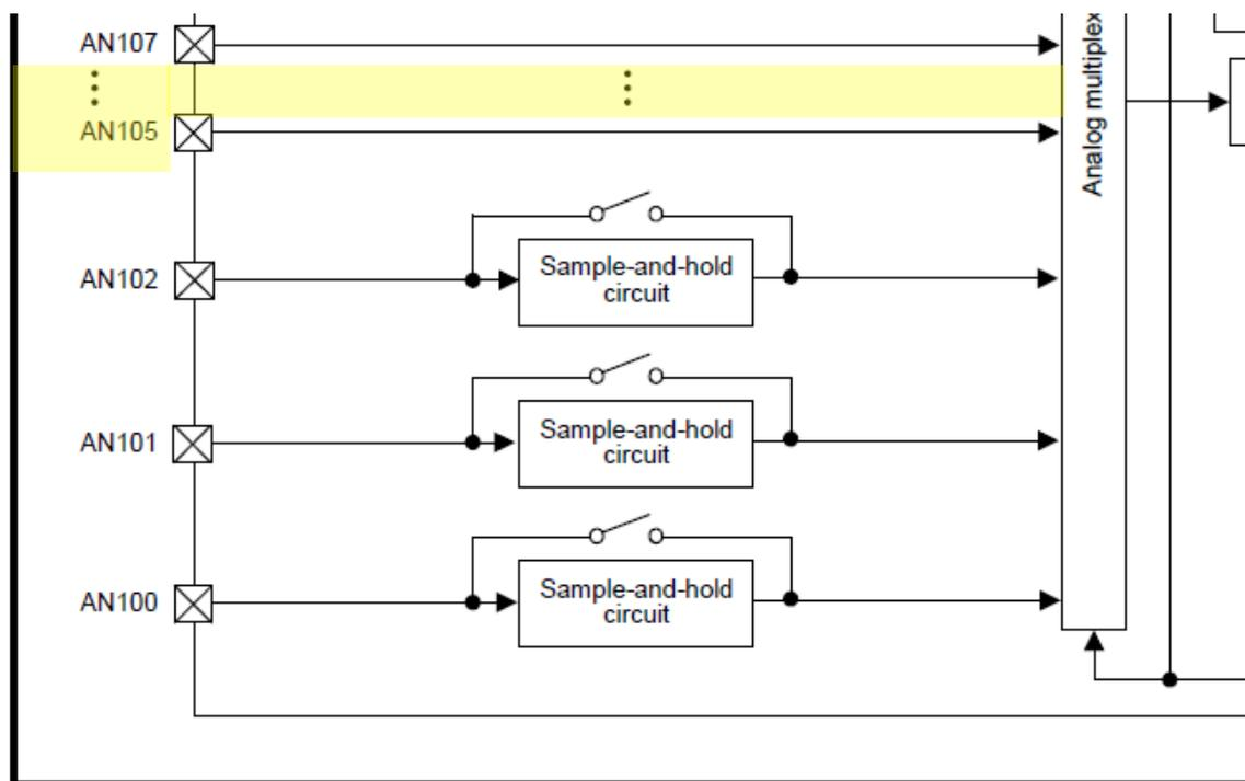
**Figure 45.2 ADC12 unit 1 block diagram**
