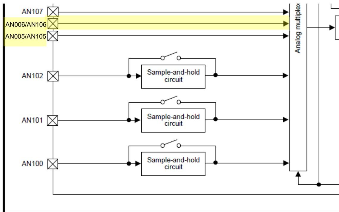
**Figure 45.2 ADC12 unit 1 block diagram**
