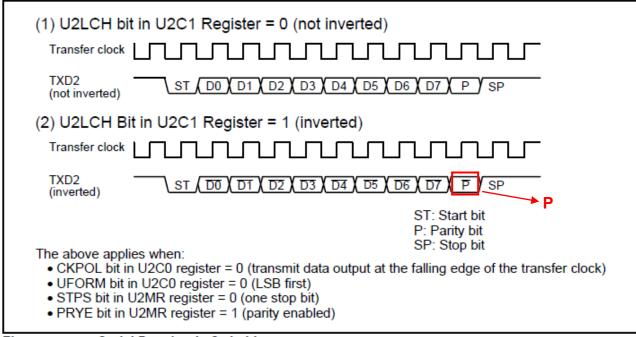
Figure Serial Data Logic Switching
