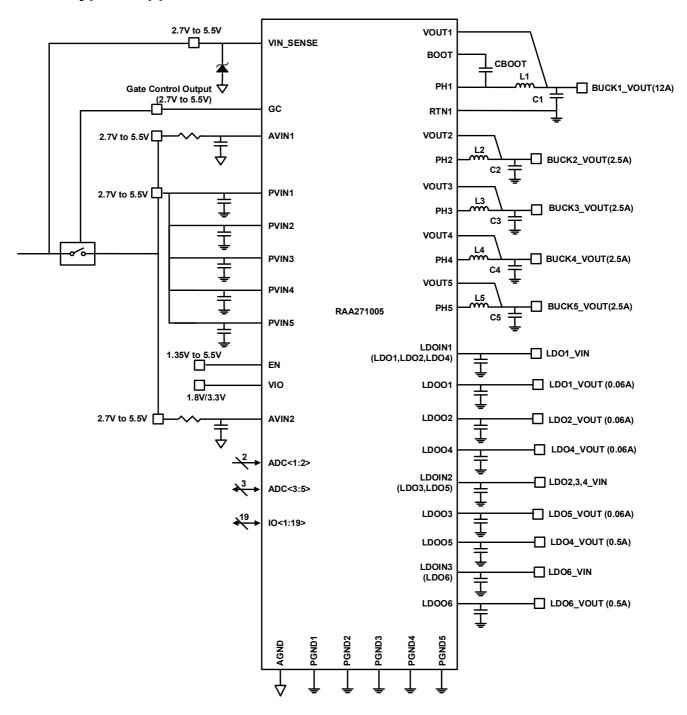
Figure 1. Typical Application with 5 Bucks
