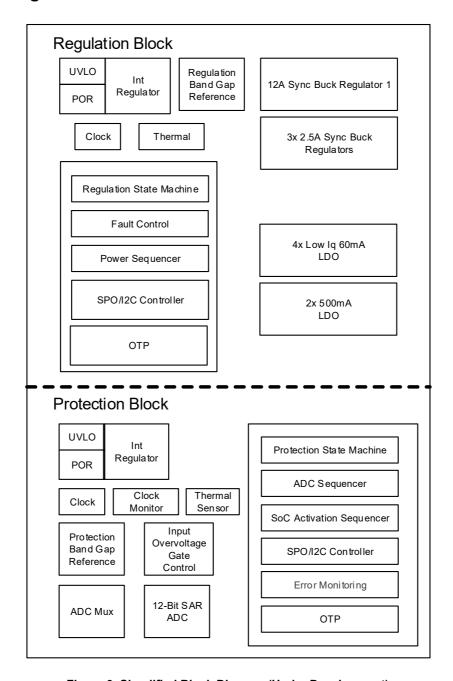
Figure 3. Simplified Block Diagram (Under Development)
