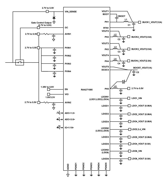
Figure 2. Typical Application with 4 Bucks + 1 Boost
