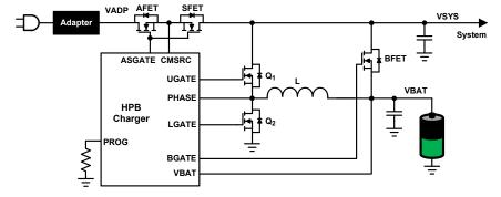
Figure 1. HPB Charger Configuration
