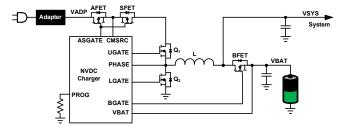
Figure 2. NVDC Charger Configuration
