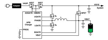
Figure 1. HPB Charger Configuration
