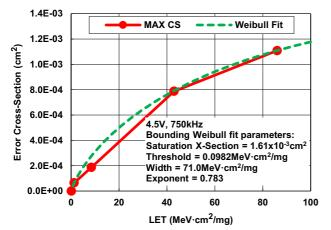
Figure 8. SET Cross-Section Test Condition #2 April 2020
