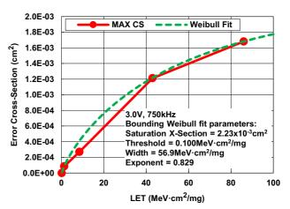
Figure 7. SET Cross-Section Test Condition #1 April 2020
