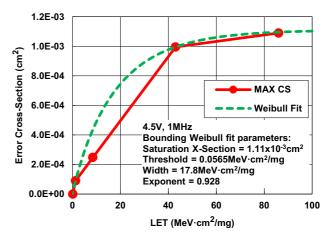
Figure 9. SET Cross-Section Test Condition #3 April 2020
