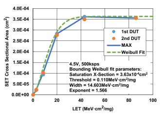
Figure 5. SET Cross-Section Test Condition #2 September 2019
