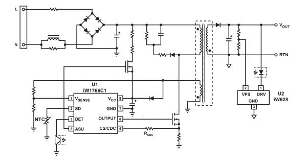
Figure 3.2: iW628 Typical Application Circuit (Using iW1766C1 as Primary-Side Controller) (Achieving < 10mW No-Load Power Consumption in 5V2A Adapter Designs with Fast Dynamic Load Response)
