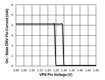
Figure 7.2 : On-State DRV Pin Sink Current (V<sub>DRV</sub>=3.5V) vs. VPS Pin Voltage
