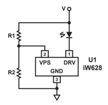
Figure 3.1: iW628 Typical Application Circuit (LED is on when  $V_{VPS}$  < internal  $V_{REF}$ )
