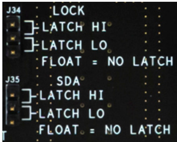
Figure 7. Lock Pin and SDA Pin Latch Control
