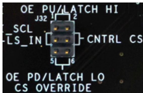
Figure 6. OE Pin Control
